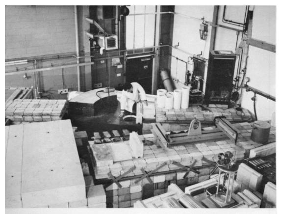
The experimental hall of the Harwell electron linac. The target is behind the shielding to the right, and the view shows the constant Q spectrometer, with the author, and the back-scattering spectrometer in the left foreground.
