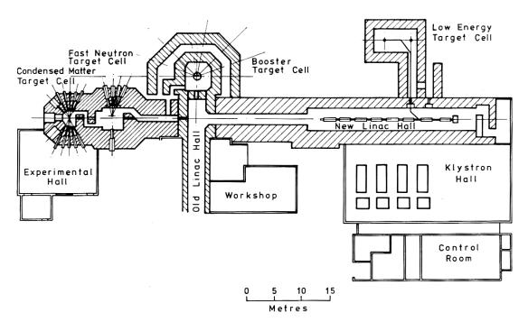
Fig. 1. Layout of the Harwell 136 MeV electron linac. The 'Old Linac Hall' housed the 1959 ~50 MeV electron linac which fired straight ahead into the Neutron Booster Target (NBT). Although only one experimental hall was originally built for condensed matter studies, another experimental hall was soon built on the other side of the Condensed Matter Target (CMT) Cell.
