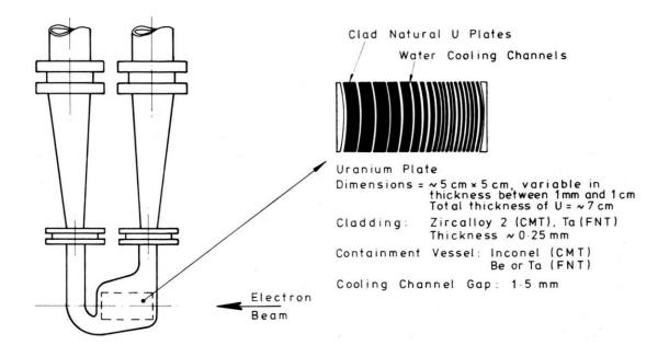
Fig. A2. Details of the Condensed Matter and Fast Neutron Targets. Calculations and measurements made in connection with the design of these targets benefited the designs of the ISIS targets. The targets could be raised remotely into a heavily shielded 'attic' to allow personnel access to the target cells.
