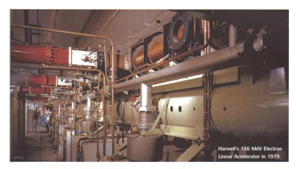
Fig. 2. The Harwell 136 MeV electron linac, inside the linac hall, looking upstream<sup>6</sup>.
