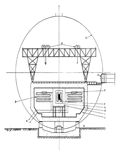
An advanced type of atomic reactor at Dounreay which is designed to produce more nuclear fuel than it consumes, while at the same time providing substantial quantities of heat energy for the generation of electricity. As an additional safety measure it is enclosed in a great sphere of steel made of plates one inch thick.
