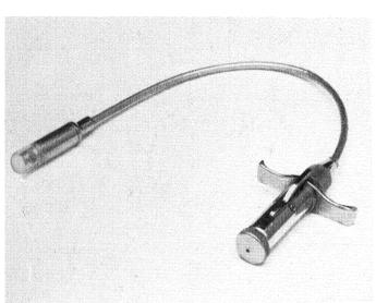
18. A "vest pocket" source of X-ravs capable of being introduced through the mouth or through surgical incisions. The source, no bigger than a cigarette end, is only exposed when the plunger at the other end of the cable is depressed.
