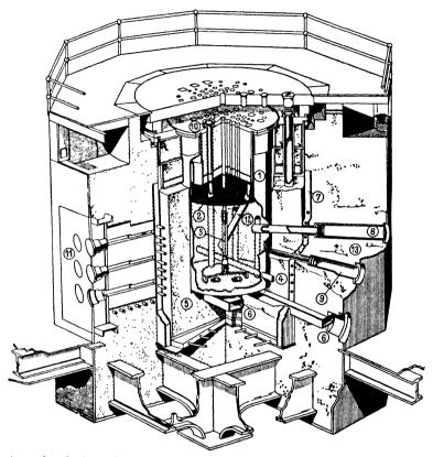
A sectional view of the heavy water reactor Dido at the Atomic Energy Research Establishment, Harwell. Jobs which took a year to do in earlier British reactors can be performed by Dido in a fortnight.
