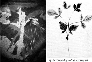
22. A radioactive crystal of the metal zirconium, photographed through a microscope by means of television to see what damage it has suffered by a period of irradiation in an atomic reactor.
