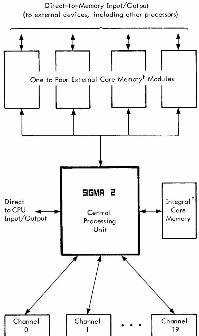
Automatic Input/Output Channels (4 standard, up to 20 total - all operating simultaneously)
