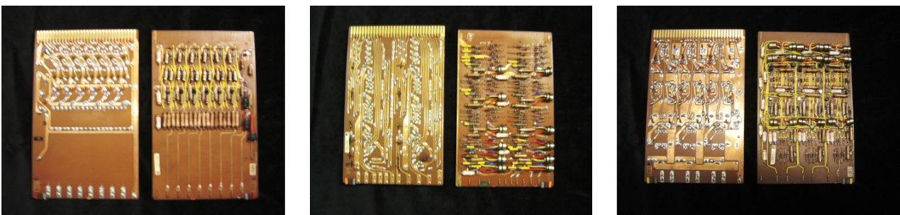
Figure 14. The front and back of three sample Atlas printed-circuit boards from bay 2 of the CPU cabinet. (From left-to-right): type 812 (adder carry), type 813 (adder input) and type 814 (adder output).
