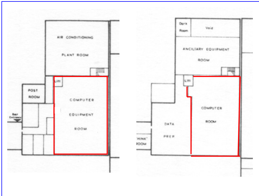
Figure 5. Part of the ground-floor plan ( left ) and first-floor plan ( right ) of the Atlas Computer Laboratory. The areas in red, each measuring roughly 50 ft. by 70 ft. (15m x 21m), housed the main functional units of Atlas.
