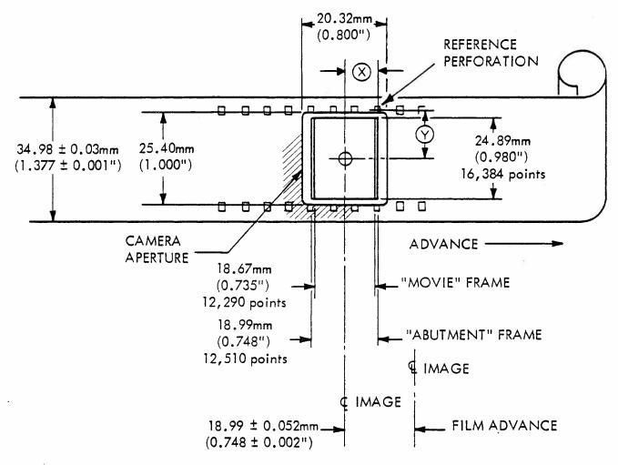
CENTER OF IMAGE TO CENTER OF REFERENCE PERFORATION: 11.88 ± 0.08mm (0.468 ± 0.003") REPEATABLE WITHIN ±0.01mm (±0.0004").
