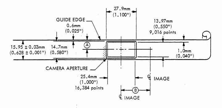
$\overset{\text{CENTER OF IMAGE TO GUIDE EDGE OF FILM: 7.98 \pm 0.13mm (0.314 \pm 0.005")}}{\text{REPEATABLE IMAGE TO IMAGE WITHIN \pm 0.04mm (0.0015")}}.$
