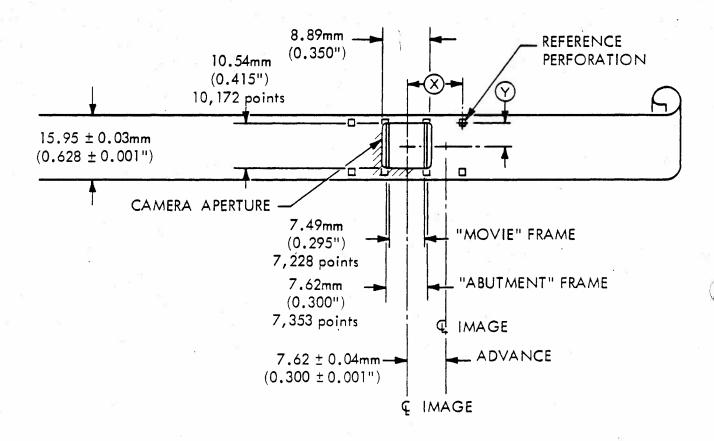
CENTER OF IMAGE TO CENTER OF REFERENCE PERFORATION: 11.43 ± 0.06mm (0.4500 ± 0.0025") REPEATABLE WITHIN ± 0.01mm (±0.0004").
