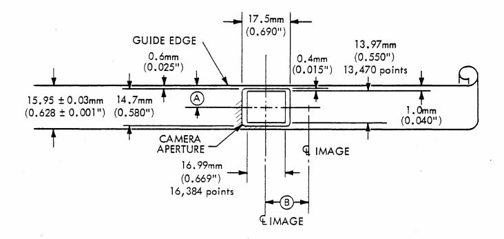
CENTER OF IMAGE TO GUIDE EDGE OF FILM:  $7.98 \pm 0.13$ mm ( $0.314 \pm 0.005$ ") REPEATABLE IMAGE TO IMAGE WITHIN  $\pm 0.04$ mm (0.0015").
