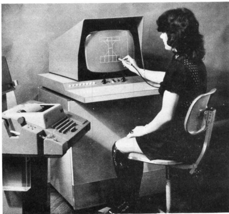
Figure 2: ICL 4280 refresh display terminal with lightpen (and foot pedal), function buttons and keyboard
