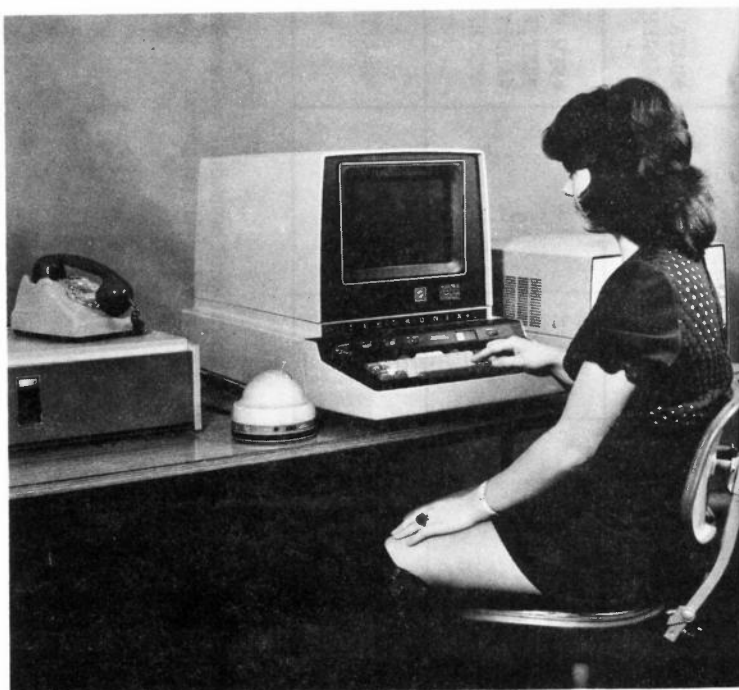
Figure 3: Tektronix 4002A storage tube display with joystick, keyboard and hard copy unit
