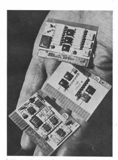
2 Unencapsulated integrated-circuit modules using special Motorola e.c.l. on single silicon chips
