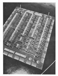
3 12-layer platter loaded with circuit modules
