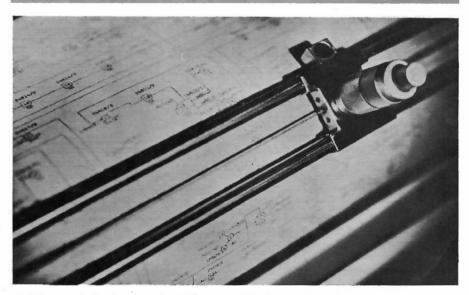
9 Calcomp plotter drawing a logic diagram online from a computer
