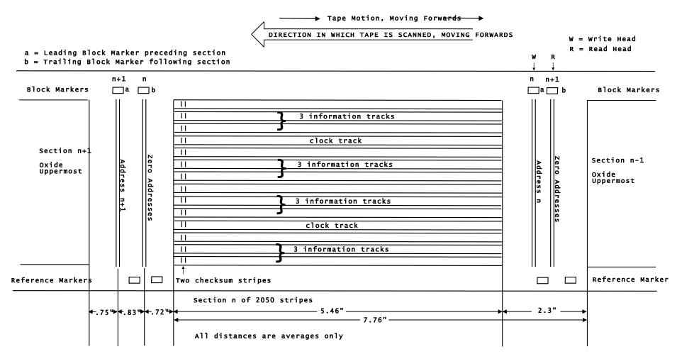
When moving forwards the tape moves from left to right, and is therefore scanned from right to left
