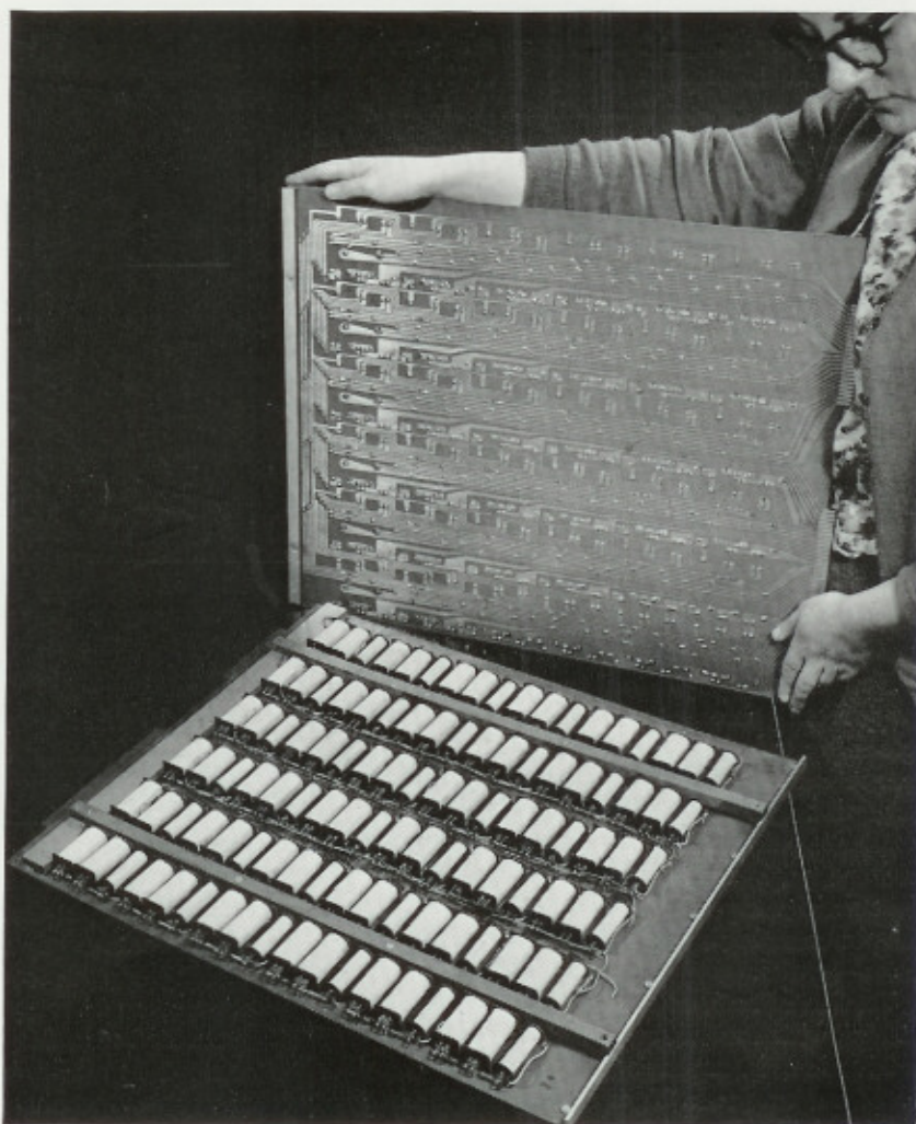
5 Printed Circuit boards from which the relay matrix is built up
