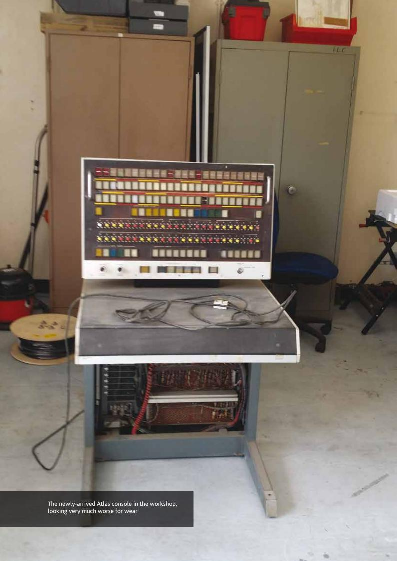
The plastic end caps were covered in black grease as though someone had repaired their car and then rearranged the caps without bothering to wash their hands first. A few of the plastic end caps were missing, damaged, or just crumbled away so replacement red and yellow versions were made. There is a single white end cap which was the most satisfying to clean, and which seems undamaged.
