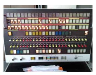
Console part-way through re-wiring. The covers have been removed from buttons we wanted lit so that new bulbs could be inserted, but it is not just these which are on!
