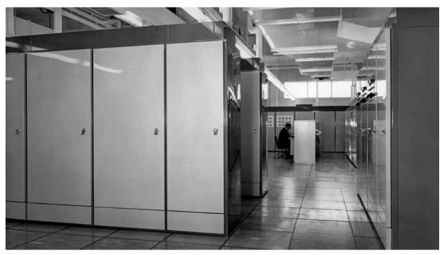
The Atlas machine room seen from the other end of the room. The power supply and switching units are on the right of the picture; core store cabinets are on the left.
