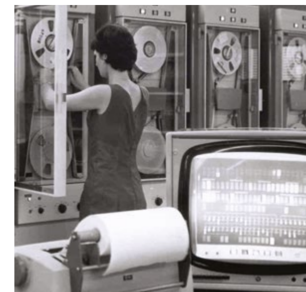
Mounting an Ampex tape. An image of the Engineer's console downstairs is shown on the monitor.
