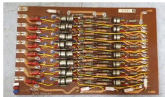
Packages: Atlas comprised about 5660 hand-soldered circuit boards or Packages, of several dozen different types. This is Package 926 from the console so is probably part of a device driver. Note that it contains Mullards – a type of transistor based on germanium rather than the faster silicon. Each package had a different function such as adder-input, inverter or flip-flop, and the different functions were indicated by three coloured tabs in the corner. Slots in the racking were marked with the same colours so that if a board was removed it could be replaced in the correct position.
