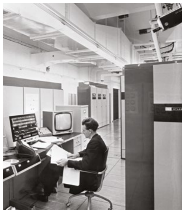
David Burrell at the Engineer's console in the Atlas machine room. To his left is a hardcopy teleprinter and paper tape reader; to his right is a CCTV monitor trained on the tape units upstairs. Behind the console are the power supply units, and behind the engineer are some of the fixed store and CPU cabinets.
