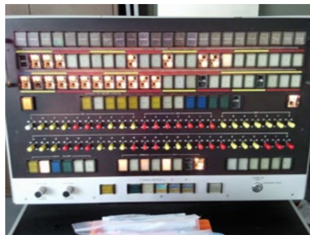
Console part-way through re-wiring. The covers have been removed from buttons we wanted lit so that new bulbs could be inserted, but it is not just these which are on!
