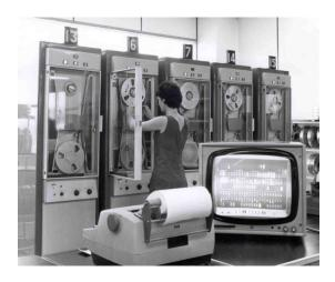
Eileen Perkins loads one of Ampex magnetic tapes in the Atlas Operations Room; in the foreground is a teletype printer and a CCTV image of the Engineer's console downstairs, 1968
