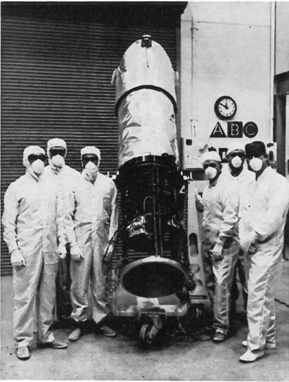
International Ultra-Violet Explorer scientific instrument. The instrument consists of a 45 cm diameter F/15 Ritchey-Chretien telescope, which collects radiation from astronomical sources and directs this to one of the two spectrographs. There a spectrum of the input radiation is recorded by a UV-sensitive television camera and converted to video signals for Telemetering to the ground. There are two UV cameras in each spectrograph—one 'prime' and one 'back-up'
