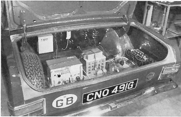
Signal conditioning equipment and instrumentation power supplies are carried in the luggage compartment of the test vehicle
