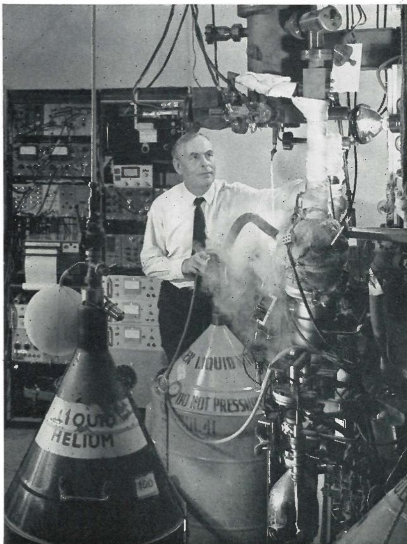
Len Gowland, UKAEA Culham, gets to grips with the ‘hissing, clicking and clattering mass of pipes, wires and meters’ that refrigerate and reduce gas density at temperatures down to absolute zero ( -273^{\circ}\text{C} ). As described in the article (begin on p. 9), it was used recently by Dr Terry Lee and a team from ROE to simulate interstellar space.
