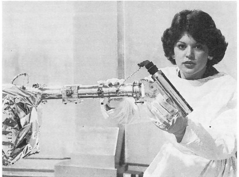
This section of a radial boom on the GEOS satellite shows (left) a magnetometer that will measure the magnetic field in three axes so enabling its precise direction to be determined at any time. An electron gun (right)—one of four on-board GEOS—will emit an electron beam which after deflection by the magnetic field is sensed by another part of the experiment—so allowing electric field components to be measured.
