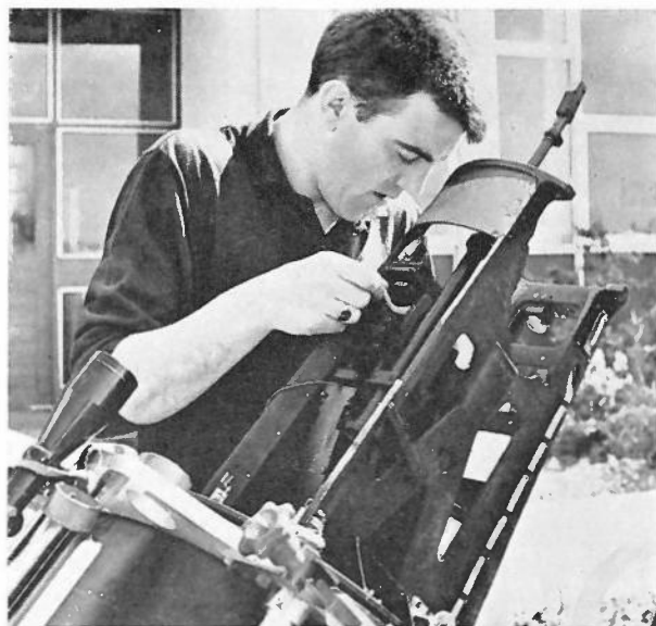
Sunlight testing of spectrographs of a Skylark rocket payload assembly.
