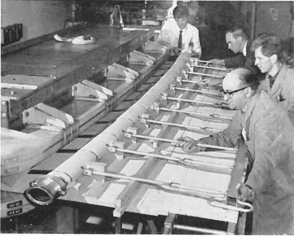
Installation of the first 'D' type ceramic vacuum chamber in a magnet at Daresbury. The individual ceramic sections can be seen making up the curved chamber with its metal end flanges.
