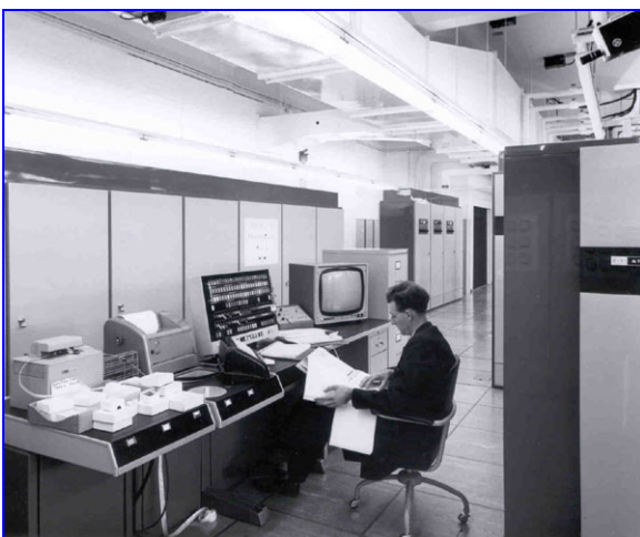
Fig. 7. These two views of an engineer sitting at the console of the Chilton Atlas give an idea of the size of the machine room. Input/output equipment was in the room directly above – (see Fig. 8).
