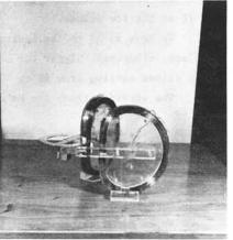
To measure the different angles mutual inductances a volt-amperometric method has been used.
