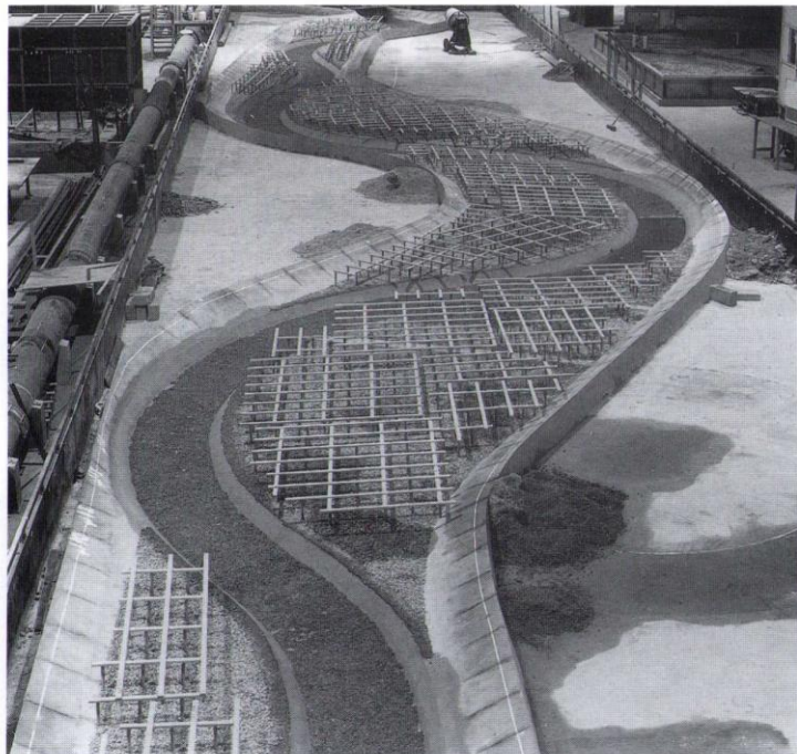
The SERC Flood Channel Facility at HR Wallingford showing a model two-stage meandering channel used during the River Blackwater study. (photo: HR Wallingford)
