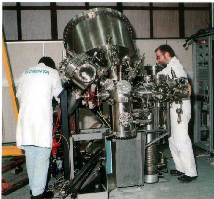
The ES300 spectrometer being installed at RUSTI by SCIENTA engineers.
