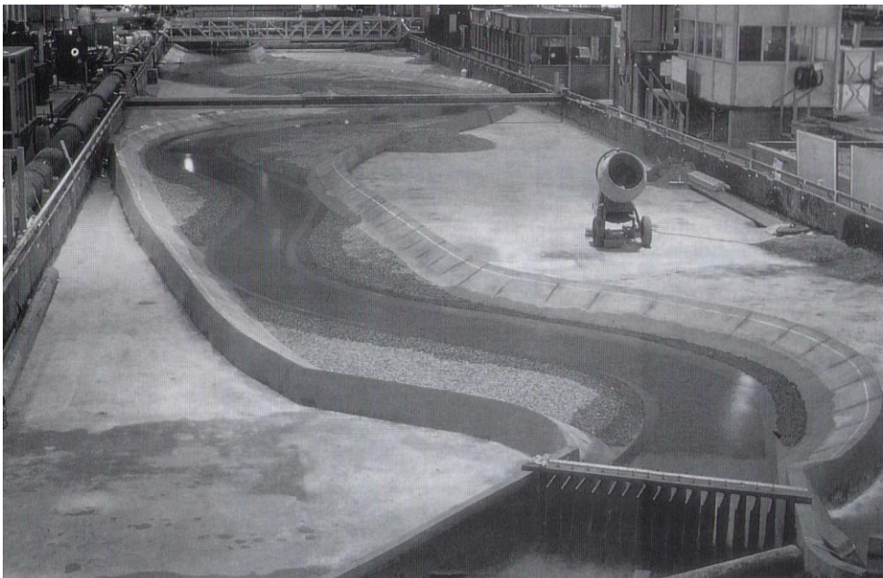
Modelling the flow of water over floodplains roughened with an array of vertical rods was an important component of the Blackwater study. (photo: HR Wallingford)
