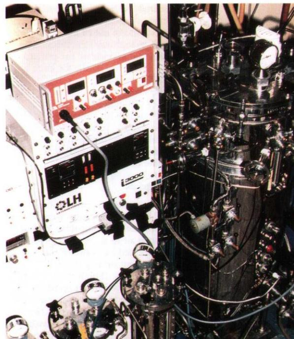
A biosensor in the research environment — an Aber Instruments "Bugmeter" in use at UCL Department of Biochemical Engineering. The Bugmeter was developed with Biotechnology Directorate support.
