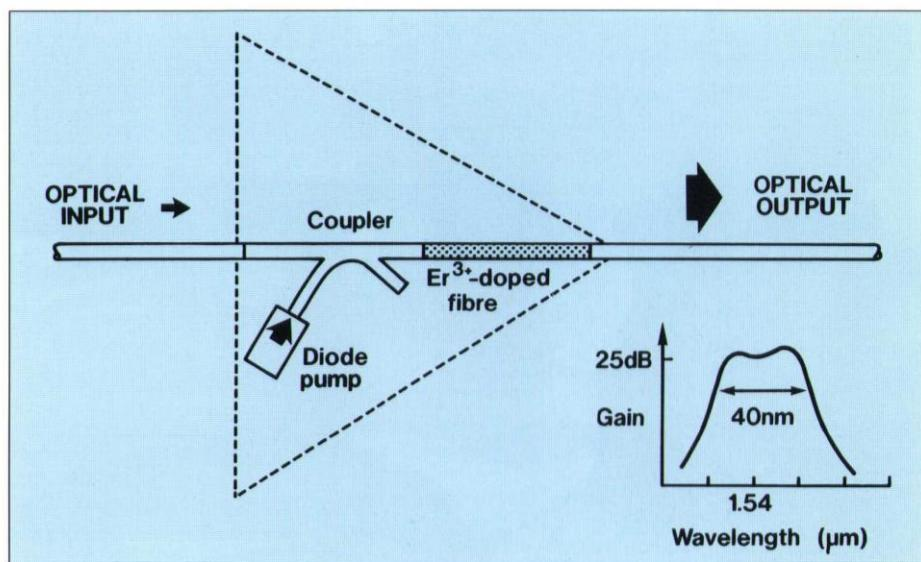
Schematic diagram of an optical fibre amplifier. The input signal, along with pumping radiation, enters one end of the doped fibre and is amplified during propagation along it. The combination of fibre coupler and doped fibre is spliced into the main fibre transmission line. Gains of over 50dB (x100,000) can be obtained. A linewidth of 40nm corresponds to a bandwidth of 5000GHz.
