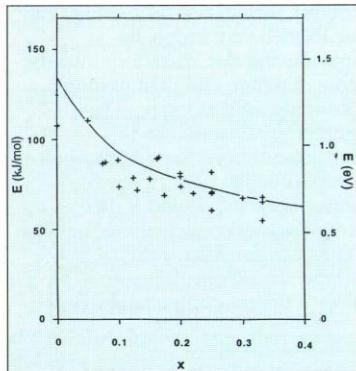
Figure 5: Activation energy for sodium diffusion in sodium silicate glasses.
