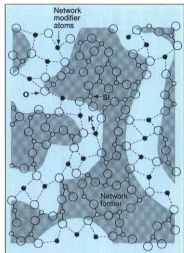
Figure 3: Schematic of Modified Random Network.
