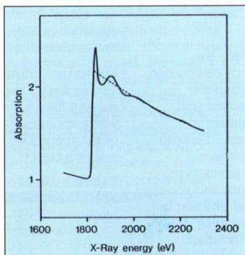
Figure 2: EXAFS at the K-edge of silicon in glass.
