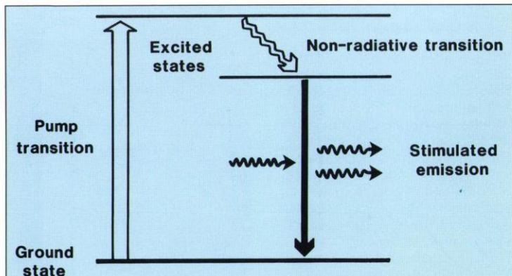
Simplified energy level diagram of the erbium ion. Radiation at the pump wavelength raises the ion energy into a range of excited states which decay rapidly to a metastable level. An input photon of the appropriate wavelength can stimulate a transition back to the ground state with the associated creation of a second photon of equal wavelength and phase.
