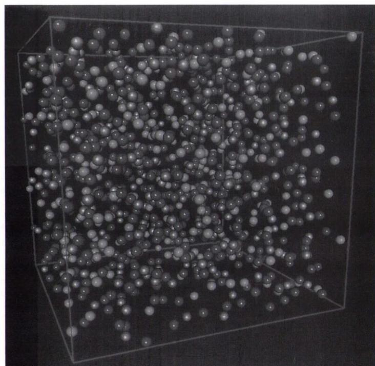
Figure 4: Molecular dynamics calculation of the structure of a sodium disilicate glass.
