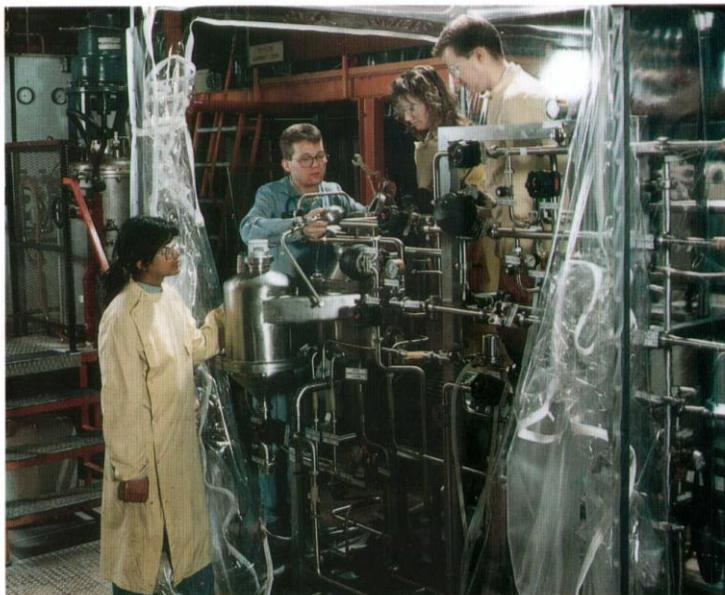
A high-speed stream-sterilisable centrifuge on test for biocontainment before installation in the Advanced Centre for Biochemical Engineering, at the UCL IRC.
