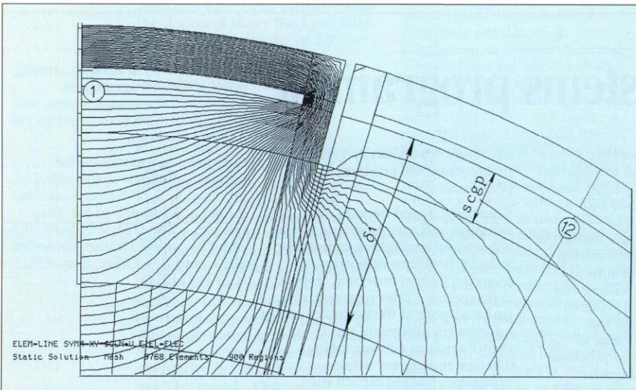
Figure 2: CAD study of electric field distribution around inter-electrode radial guard screens, important in reducing the standing capacitance between adjacent electrodes.
