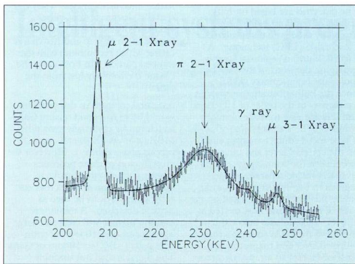
Figure 2: The  $22\text{ Ne}$   $\pi^-$  X-ray spectrum measured at TRUMF
