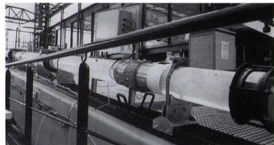
Figure 5: The sensor system in place in the inclinable multi-component flow investigation loop at Schlumberger Cambridge Research, which allows controlled mixtures of oil and gas to be pumped through the sensor section over a range of flow rates and under a variety of flow regimes.
