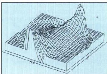
Figure 3: Example of capacitance sensitivity distribution, for diagonal electrode pair (1-7).
