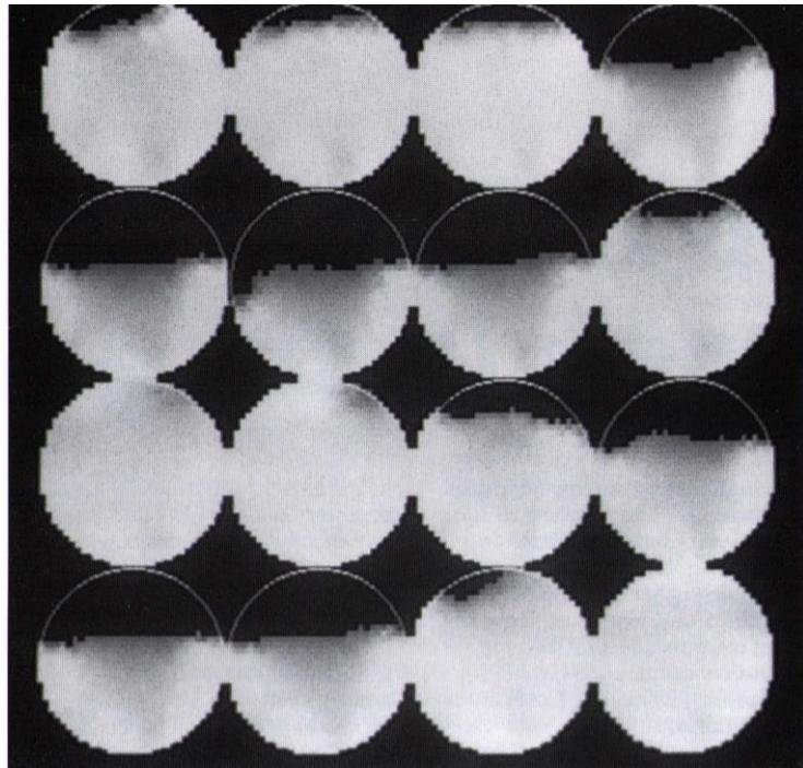
Figure 4: Typical experimental results. From top to bottom, left to right, the picture shows the development of gas slugs of a gas/oil flow in an inclined pipe (6° from horizontal, see figure 6). Time interval between successive images is 80 ms.
