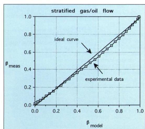
Figure 6: Calibration curve showing the actual volume fraction of oil compared with the volume fraction measured from the tomographic image for stratified gas/oil flow.
