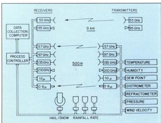
Figure 2: Block diagram of the 500 m and 9 km experimental transmission ranges at Chilbolton.
