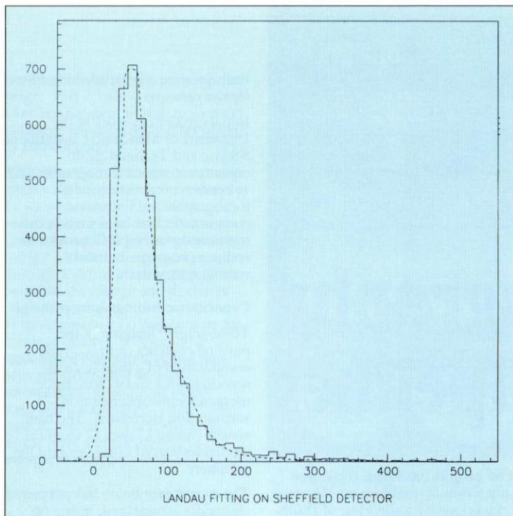
Figure 2: The figure shows the observed energy spectrum from a GaAs microstrip detector in a beam of high energy minimum ionising particles. The histogram is the data and the dotted line is the predicted spectrum due to the particles.
