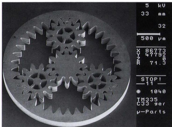
A micro-mechanical component produced by the Karlsruhe company, MicroParts, now using Daresbury synchrotron radiation as part of their LIGA production process.
