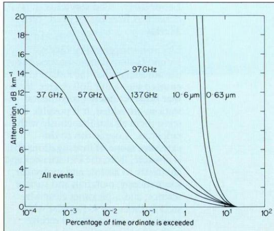
Figure 4: Cumulative distributions of attenuation measured in all types of weather over a three-year period.
