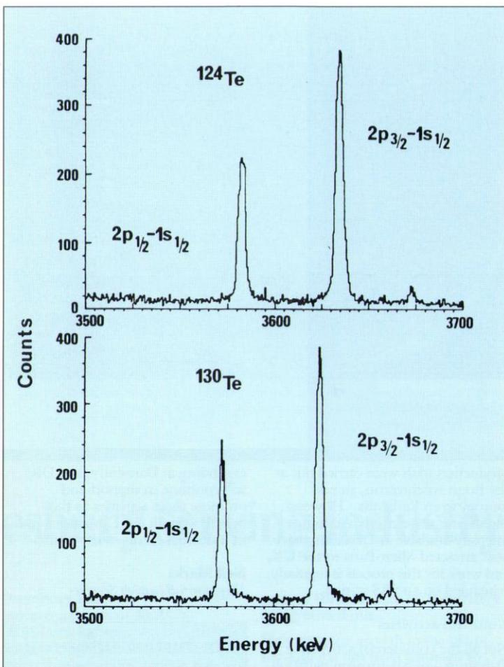
Figure 1: Muonic atom spectra for two Te isotopes measured at LAMPF. The isotope shift is about 20% of the fine-structure splitting. The measurements show that the charge radius of these isotopes differs by  $30.1 \pm 0.5 \times 10^{-18} \text{ m}$ .
