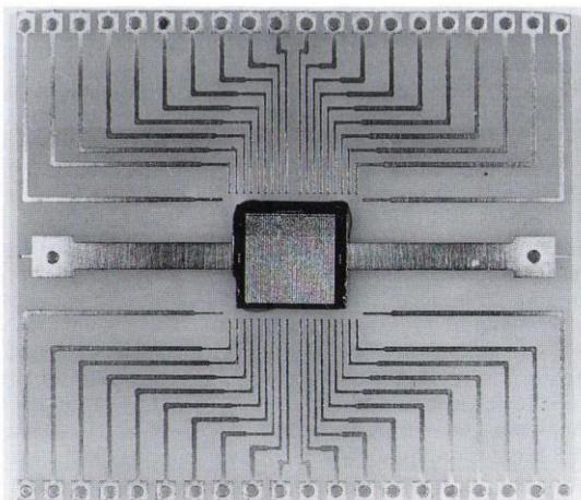
Figure 1: GaAs microstrip detector mounted on printed circuit board. The detector chip is approximately 1 cm square and has 40 microstrip devices each with an integrated bias resistor and decoupling capacitor.
