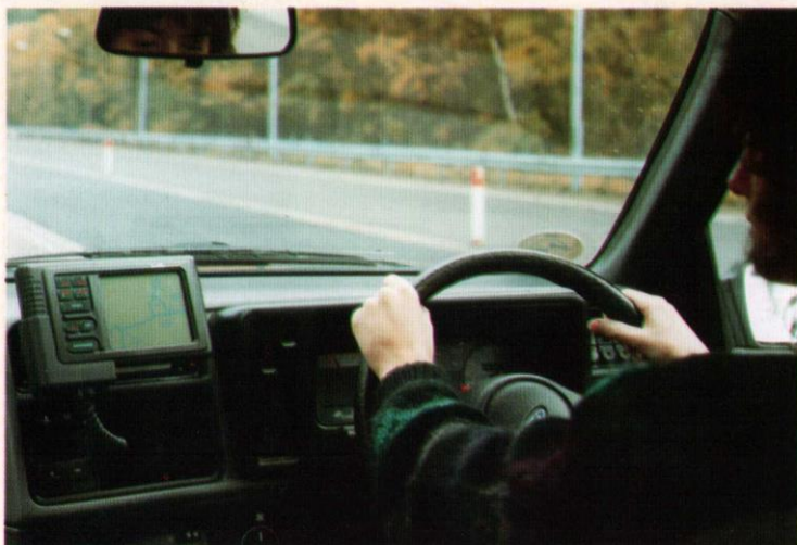
Route guidance. The system being developed by the Transport and Road Research laboratory will include a dashboard mounted visual display showing a map of the route to be taken, distance to destination and direction of travel at each junction.
