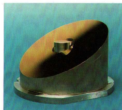
Figure 2: One of the diamond-turned optical assemblies showing an ellipsoidal collimating mirror mounted in the centre of a larger folding mirror. These mirrors are aligned using pads machined to the same precision as the optical surfaces.
