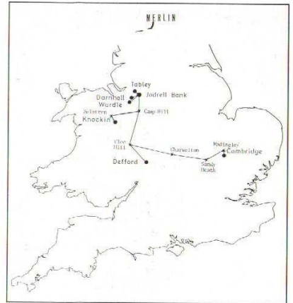
Figure 1: Map of the MERLIN array of radio telescopes linked to Jodrell Bank. The addition of the 32-metre telescope at Cambridge increases the maximum baseline to 230 km. The telescopes are shown by circles. The microwave link sites bringing the astronomy signals back to Jodrell Bank are shown by crosses.
