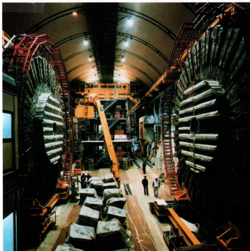
Figure 4: The Experimental Hall in Pit 8: in the foreground the two magnet end-caps and detectors; in the background, the control barracks and main body of the detector.
