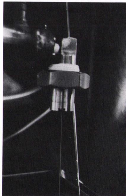
Spinning a porous hollow fibre membrane for use in gas separation. The freshly spun fibre descends through air from the spinneret into the coagulant bath. (Photo: Leeds University)
