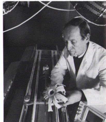
PEG-supported research in cooperation with industry has led to the development of complex composite ropes that are more durable than steel strands. Here, Professor Derek Hull is holding a partially crushed glass fibre-polyester resin tube that has been tested on his catapult crash rig at Cambridge University's Department of Materials Science and Metallurgy. (Photo: COI).
