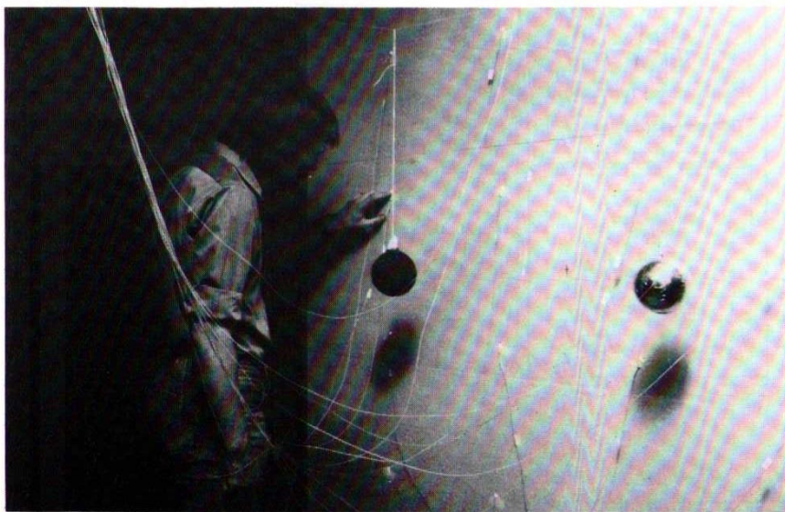
Attaching thermocouples to a test wall.
