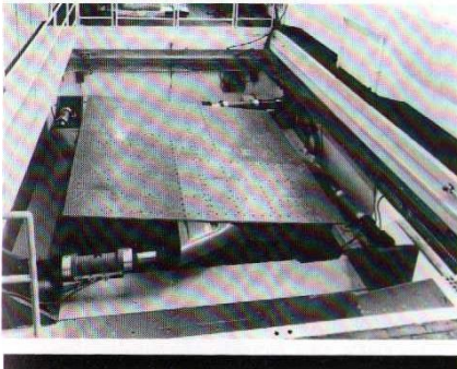
The shaking table in the 'pit', showing the four horizontal actuators.
