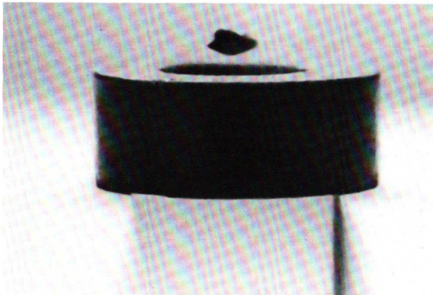
A 6mm piece of yttrium-barium-copper-oxide in the superconducting state levitated over a ring of permanent magnet material. (Photo: Cambridge University).
