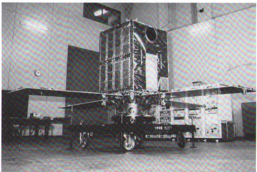
The Ginga satellite with solar panels extended. Under the eight thin thermal blanket panels that can be seen on the left side are the eight units of the LAC array. (Photo: ISAS)
