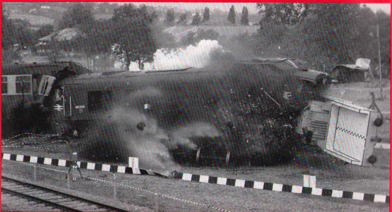
A diesel train travelling at 100 mph crashes into a nuclear fuel flask, in a demonstration by CEGB to prove the immense strength of the containers: the diesel was destroyed, the flask was unscathed. (Photo: CEGB)
