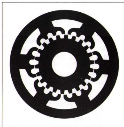
Cross-section of the laminations of a 3 kVA switched reluctance motor, showing the 24 teeth on the outer stator and the 22 teeth on the inner rotor (radial airgap enlarged for clarity). (Drawing: Newcastle upon Tyne University).
