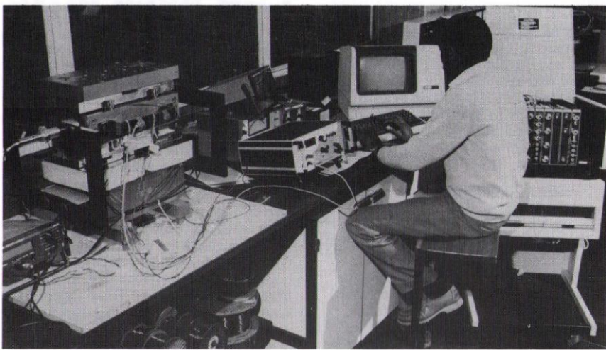
Dr Adam Musoke, Senior Research Associate with the Newcastle team, working with a linear stepping motor rig, designed for fundamental investigation of the important effects of magnetic saturation on force production between iron teeth in stepping and switched reluctance motors.
