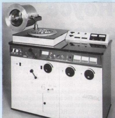
Transition metal vapour synthesis unit and (above right) details of the electron gun furnace at the heart of the machine.
