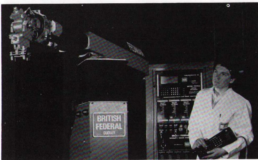
The Microman 8 microprocessor-based robot control system: a controller working with a typical robot (Photo: British Federal Ltd).
