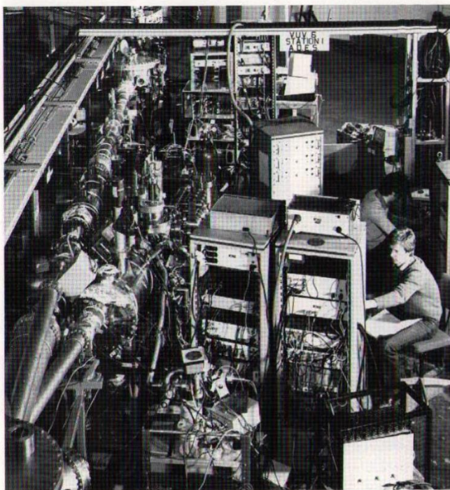
Left: A typical view of synchrotron radiation beam lines linked to experimental workstations. The storage ring is below, and to the left of the picture. The apparatus shown is for research on the properties of metal and semiconductor surfaces.
