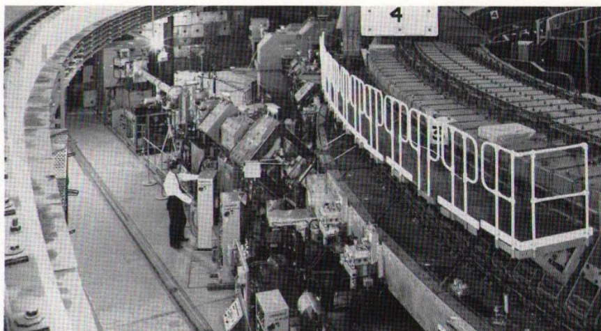
Above: part of the main ring magnet of the Nimrod proton synchrotron showing a beamline (to the left) that transports high energy particles to the experimental area.
