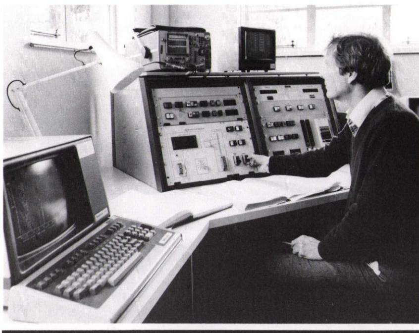
The main control station of the SLR facility. This is not usually manned during satellite ranging, because the operator must maintain a radar-assisted visual watch for aircraft from the platform surrounding the telescope. Controls and displays requiring urgent attention are duplicated.
