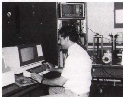
Dr David Birch of Strathclyde University operating the \gamma -ray spectrometer developed with a Cooperative Research Grant for studying how scintillation in plastics depends on the extent of polymerisation.
