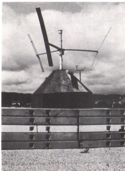
RAL wind turbine test facility, to be used in initial wind/diesel integration experiments.
