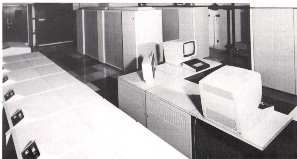
Back left: the 3081 processor (with two sliding doors) and behind it part of the processor controller. In the foreground is a row of 3350 disc drives, and back right is part of the IBM 3032.
