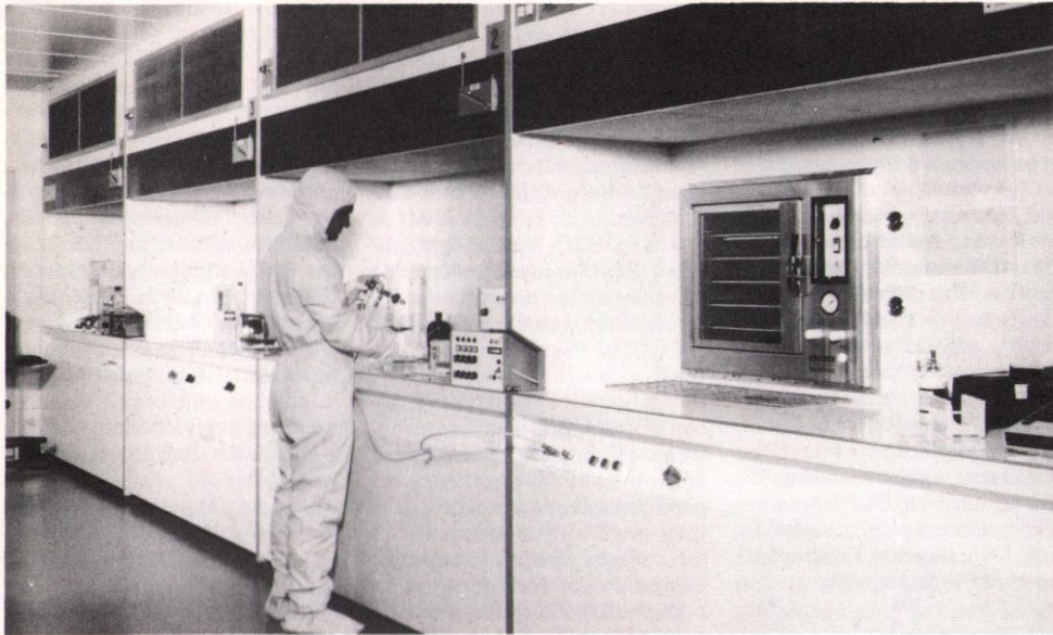
Figure 5 ▲ Part of the clean area of the EBL Facility. The operator protected by suitable clothing is preparing a plate for coating with resist.
