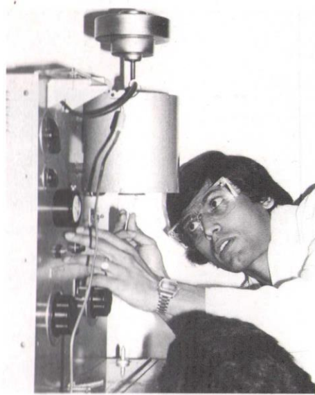
Students at the Summer School – left: measuring the melt flow index of low density polyethylene; and, right: determining polymer density using a flotation test.
