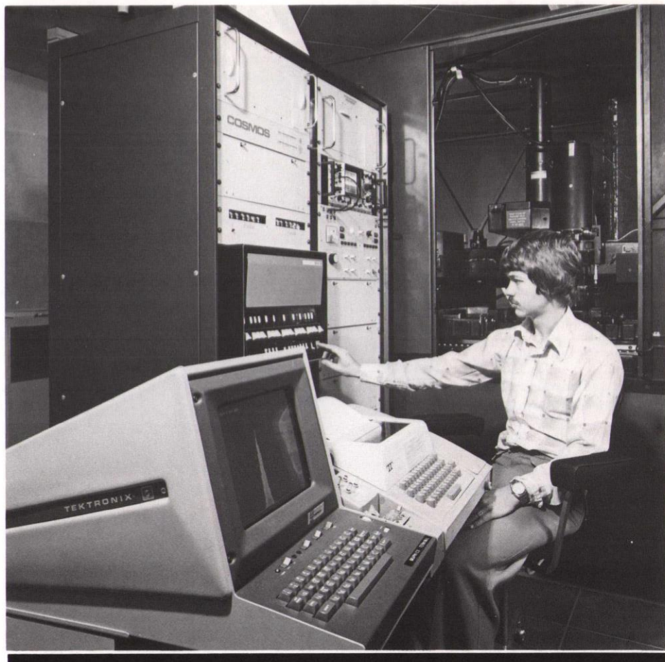
The COSMOS high-speed measuring machine at the Royal Observatory, Edinburgh is designed to extract the information contained in a photograph. At the right is the cabinet containing the basic mechanical assembly and the electro-optical components (see cover picture).
