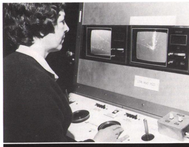
A Vanguard measuring machine for bubble chamber pictures adapted to project and digitise bubble chamber holograms. The controls allow the operator to drive the machine in three perpendicular directions and position any desired point in the bubble chamber volume under the measuring cross.
