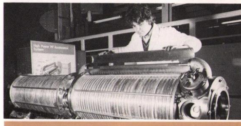
A quadrupole doublet with trim quadrupoles mounted on their base. The ceramic chamber runs through the whole unit.
