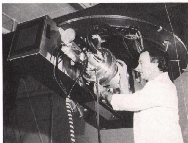
RGO design engineer D W Gellatly, with the Cassegrain spectrograph attached to the telescope simulator at the Royal Greenwich Observatory.
