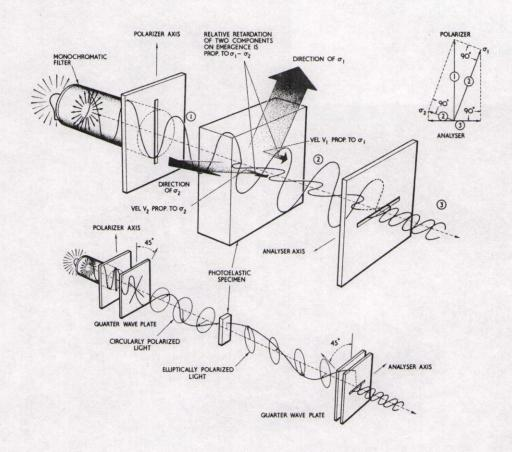
Figure 1. Principle of photoelastic stress analysis using the transmission method with a transparent specimen.
