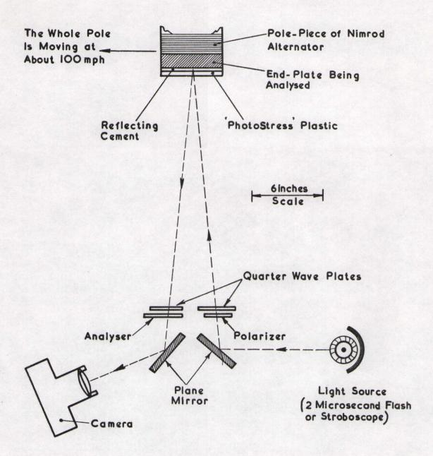
Figure 2. General arrangement of the photoelastic method used to analyse the dynamic stresses in end-plates on the main Nimrod alternators while the machines are rotating.
