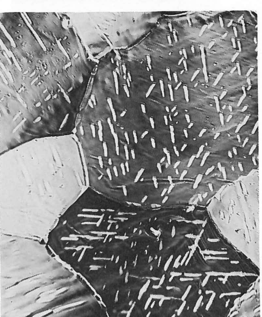
This picture shows the fine needle-like growth of tungsten carbide on a tungsten sample. The carbide was produced by the reaction of metal and acetylene gas in the microscope at 1200°C. Magnification is x 1000. Temperature 1650°C
