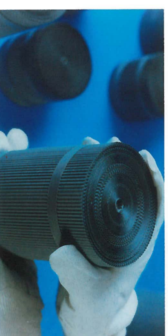
Ferrocatalyst steel coated with platinum-based catalyst for car exhaust systems. (H 48171806)
