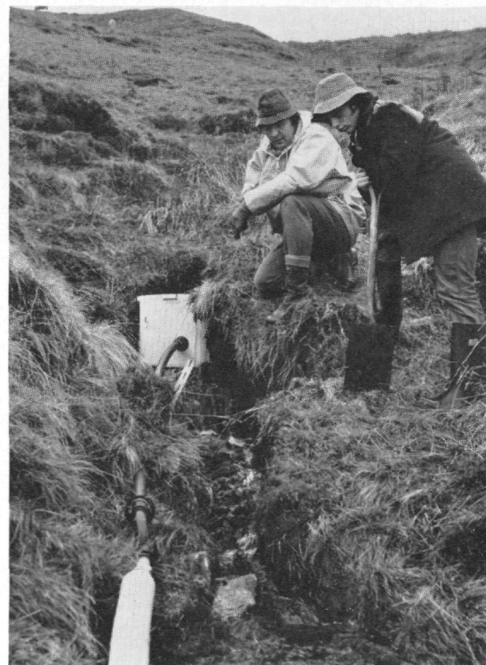
ENVIRONMENT. Airborne dust and rainwater are collected on Plynlimon, Wales, for analysis at Harwell. The station is one of seven set up in Britain for checks on the atmosphere.
