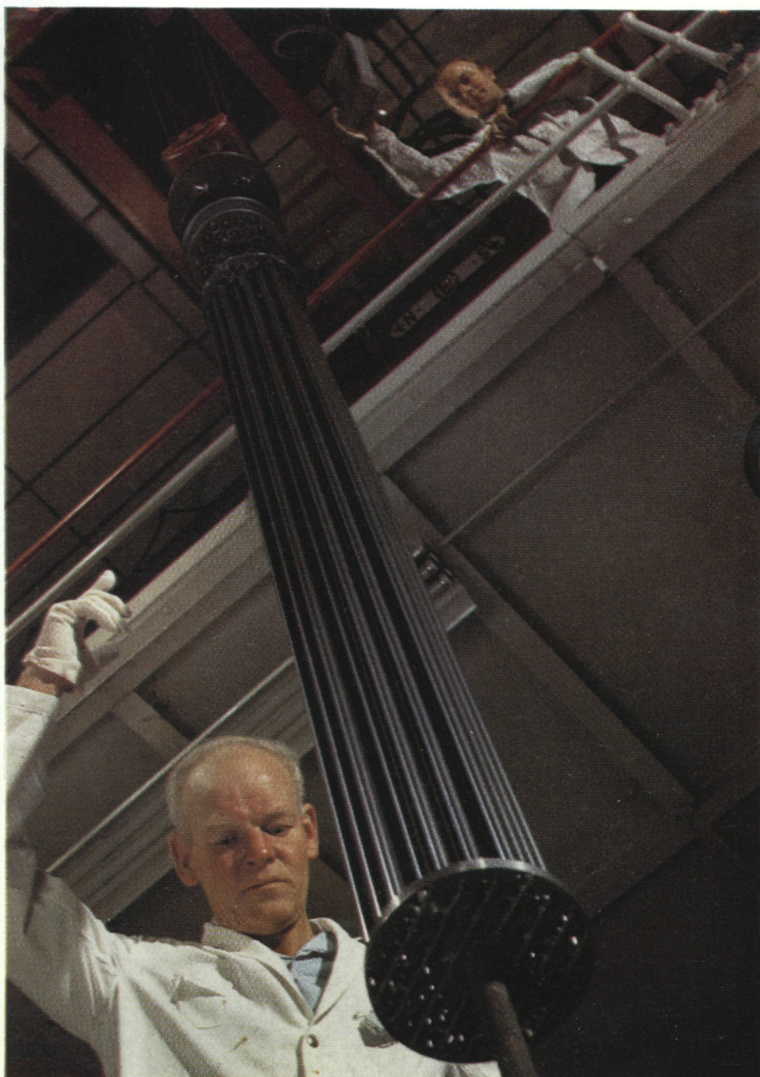
BNFL. SGHWR tubes being removed after treatment in an autoclave at the Water Reactor Fuel Plant of British Nuclear Fuels Ltd, at Springfields.
