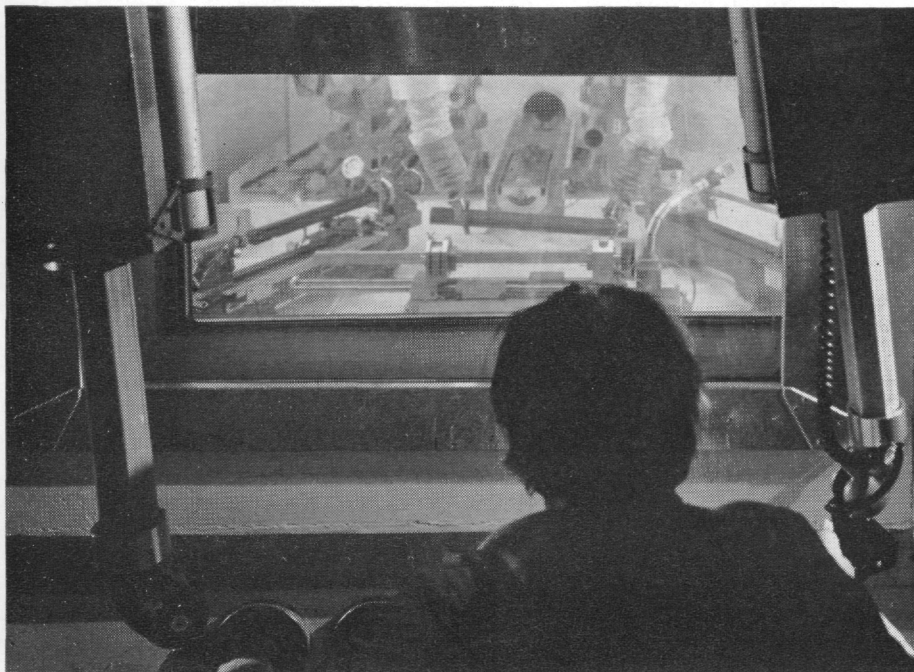
PIE. The post-irradiation examination facilities at Harwell can be applied to the fuel elements of any type of reactor.
