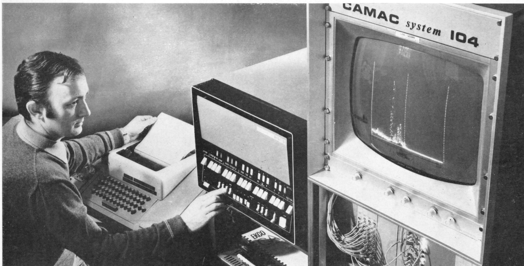
CAMAC. Harwell 7000 Series equipment conforms to the internationally agreed CAMAC (Computer-Aided Measurement and Control) specifications. Authority licensees sell the world's largest range of CAMAC-compatible equipment. Shown above is the computer-based data acquisition and display system for the analysis of nuclear events recently commissioned at the CEGB laboratories at Hornsey.
