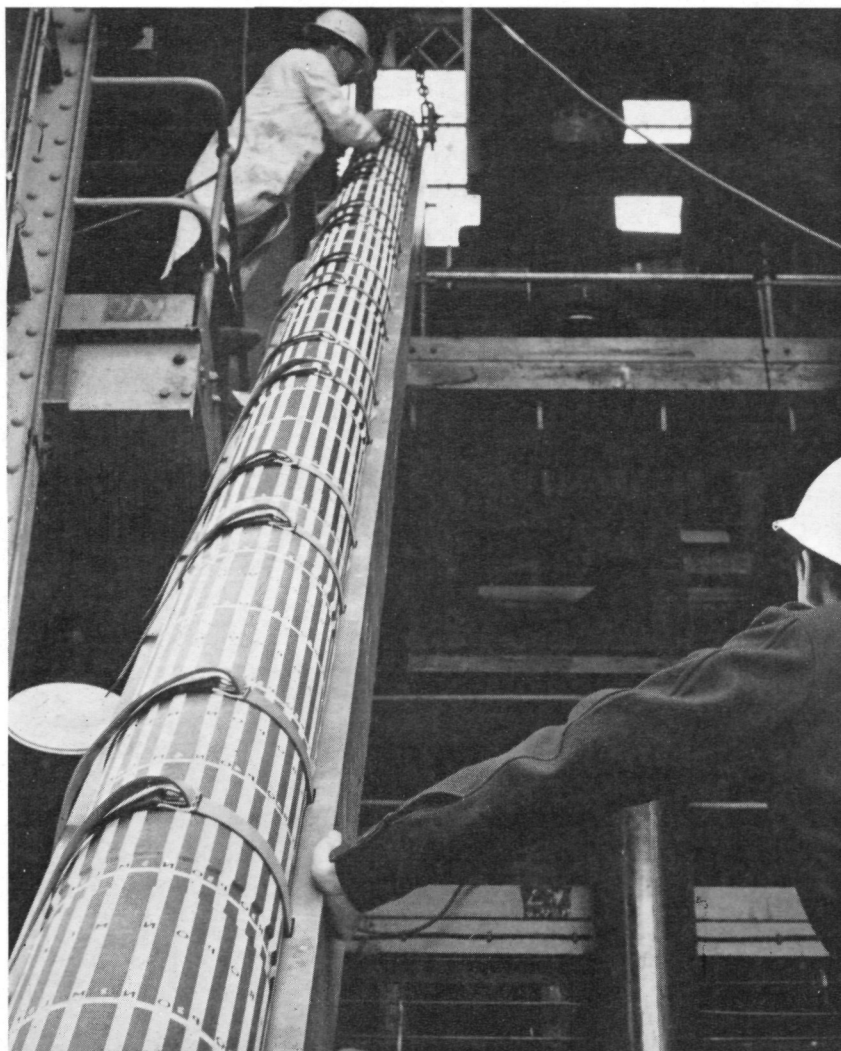
CAGR. A "stringer" of fuel elements for commercial advanced gas-cooled reactors being lifted to the vertical position in a test rig at the Reactor Development Laboratories, Windscale.
