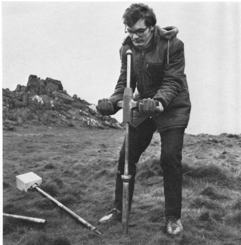
PROSPECTING. An instrument developed by Harwell and the Institute of Geological Sciences measures the radon content of sub-soil air and can locate uranium deposits too deeply buried for direct measurement of their gamma radiation. It is manufactured under UKAEA licence by Ekco Instruments, Ltd.
