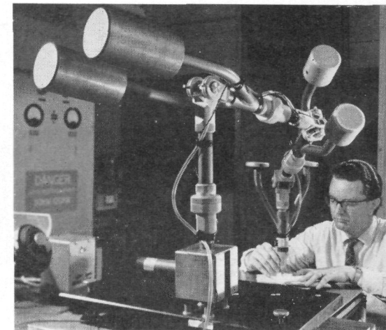
Medical Engineering. A six-joint articulated laser-beam manipulator for experimental surgery has been devised by Aldermaston.
