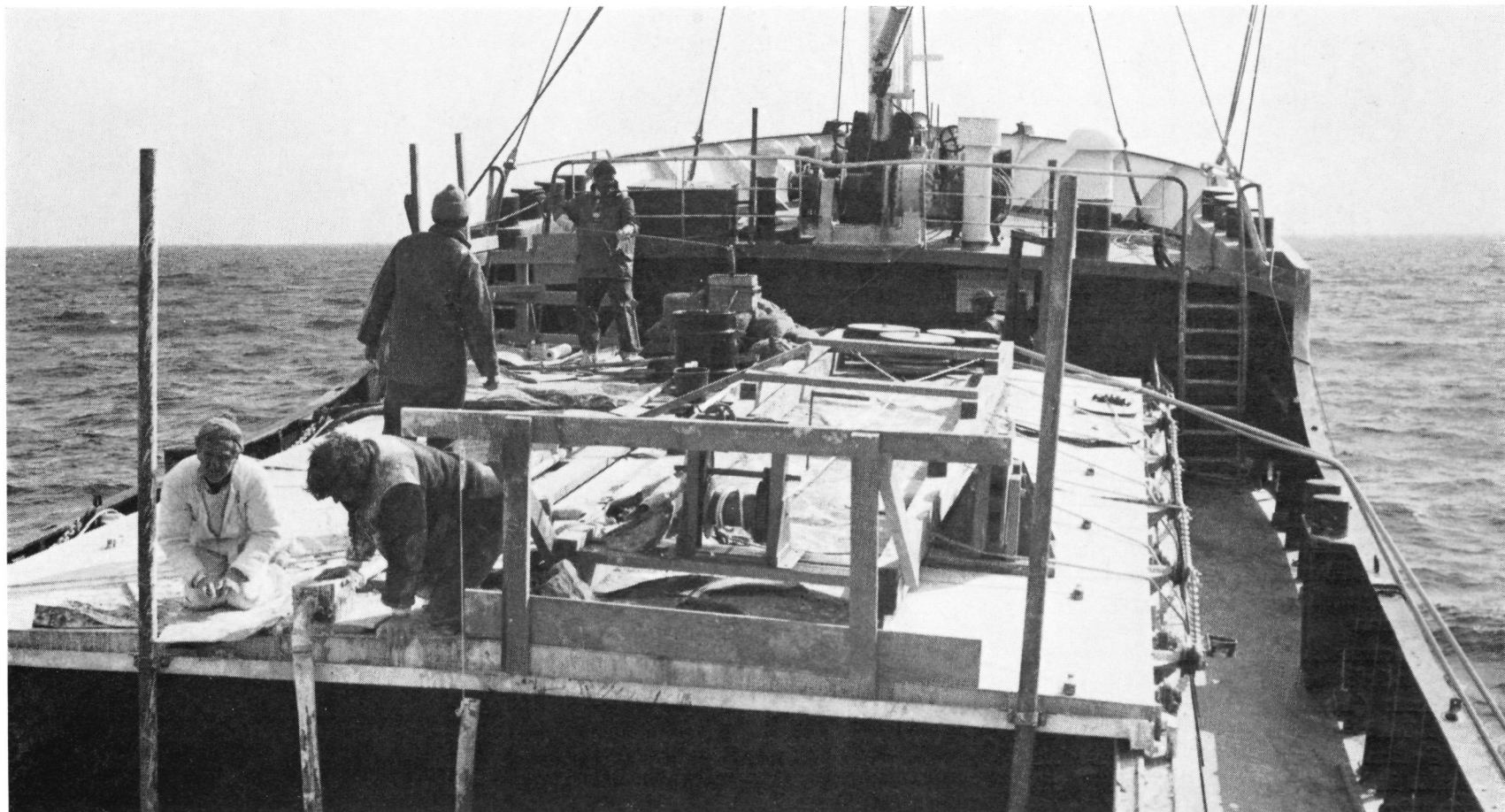
CHINA CLAY. Isotope tracers being used aboard MV "Margareta B" during experiments off Dodman Point to determine a possible position for a pipeline that could carry away waste from the Cornish china clay pits.
