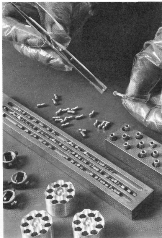
IRRADIATION. Magnesium alloy capsules being loaded with cobalt chloride pellets prior to neutron irradiation.
