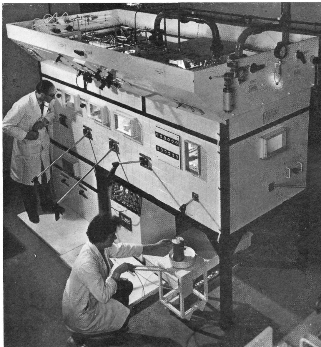
PHARMACEUTICAL DEPARTMENT. Processing iodine-125 inside a shielded cell. Improved recruitment of scientists during 1968/9 has enabled a large programme of development to be carried out in all departments.
