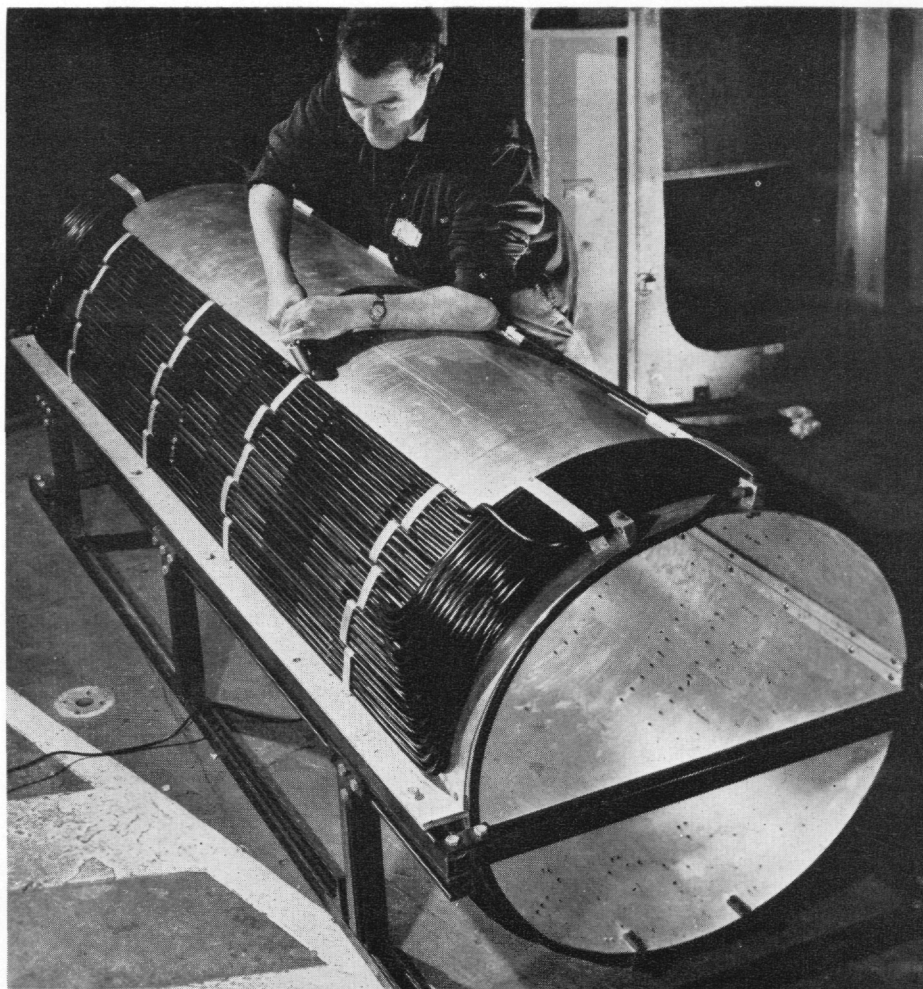
SODIUM FLOWMETER The Authority's extensive R. & D. experience on sodium cooling has been deployed to develop instrumentation for P.F.R. (whose coolant will be 1,000 tons of sodium). Above: "Saddle coil" flowmeter for measuring sodium flow in large diameter pipe.
