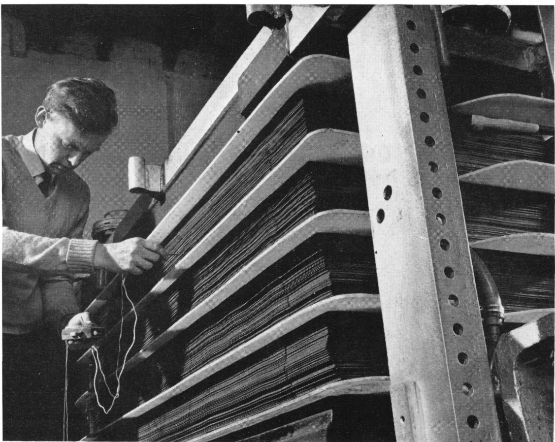
ELECTRODIALYSIS Advances developed in the 50,000 gallons-a-day pilot plant installed by William Boby & Co. Ltd., in Essex are being incorporated in the 4.2 million gallons-a-day plant they are building for Benghazi.
