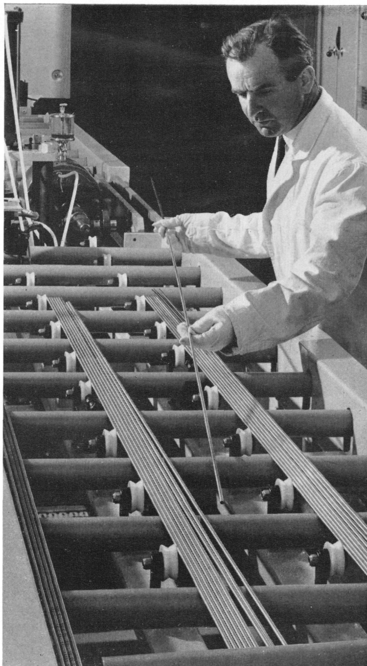
P.F.R. Swaging and cropping fuel pins for the Prototype Fast Reactor before they are loaded with fissile fuel. The Windscale plant is being used initially for P.F.R. fuel, but will have additional capacity.
