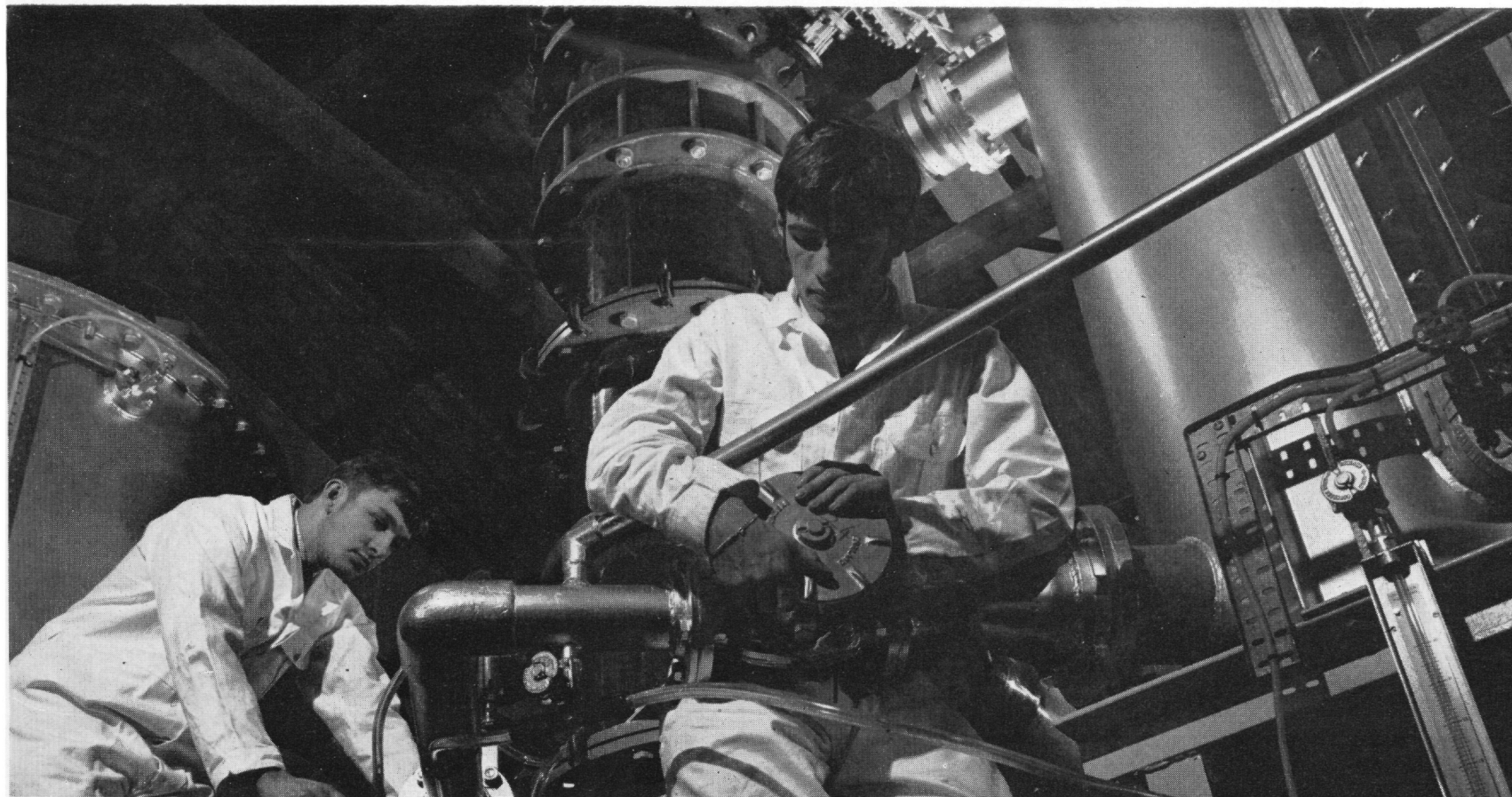
Ice crystal-brine separating column on the 10,000 gallons per day study plant for development of the secondary refrigerant (butane) freezing desalination process constructed at Simon Engineering Ltd.
