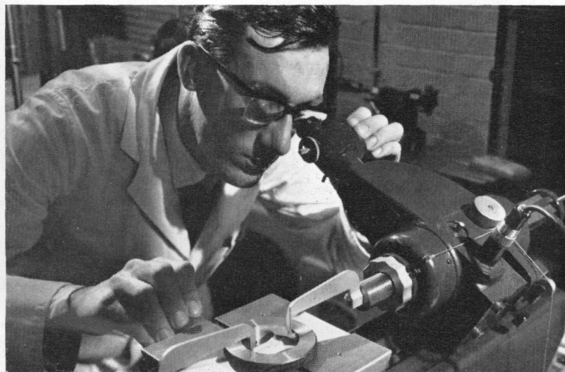
HARWELL MECHANICAL STANDARDS LABORATORY is part of the British Calibration Service, set up to test measuring instruments against approved national standards. Photograph shows calibration of a ring gauge at the Laboratory.
