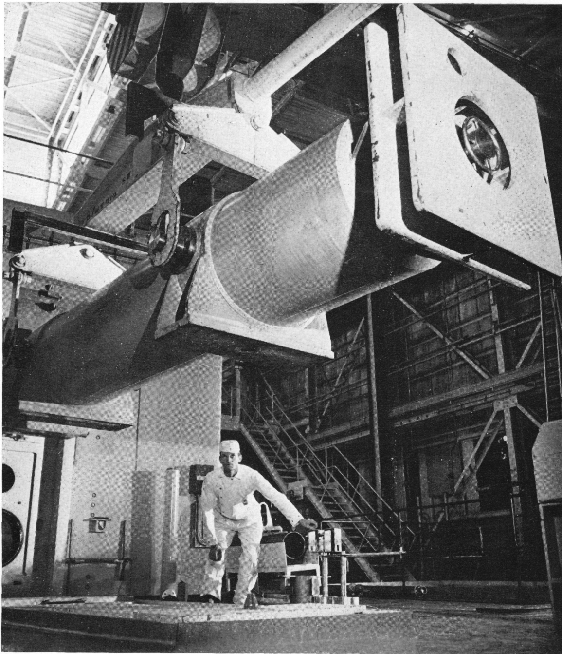
HEAD-END PLANT A new head-end plant for the primary treatment of irradiated oxide fuel is now in operation at the Windscale reprocessing plant, which has a capacity of over 2,500 tonnes a year.
