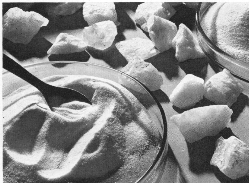
Quartz before and after it has been crushed in a Harwell rig by a shock-wave whose intensity approaches that of a chemical explosive.
