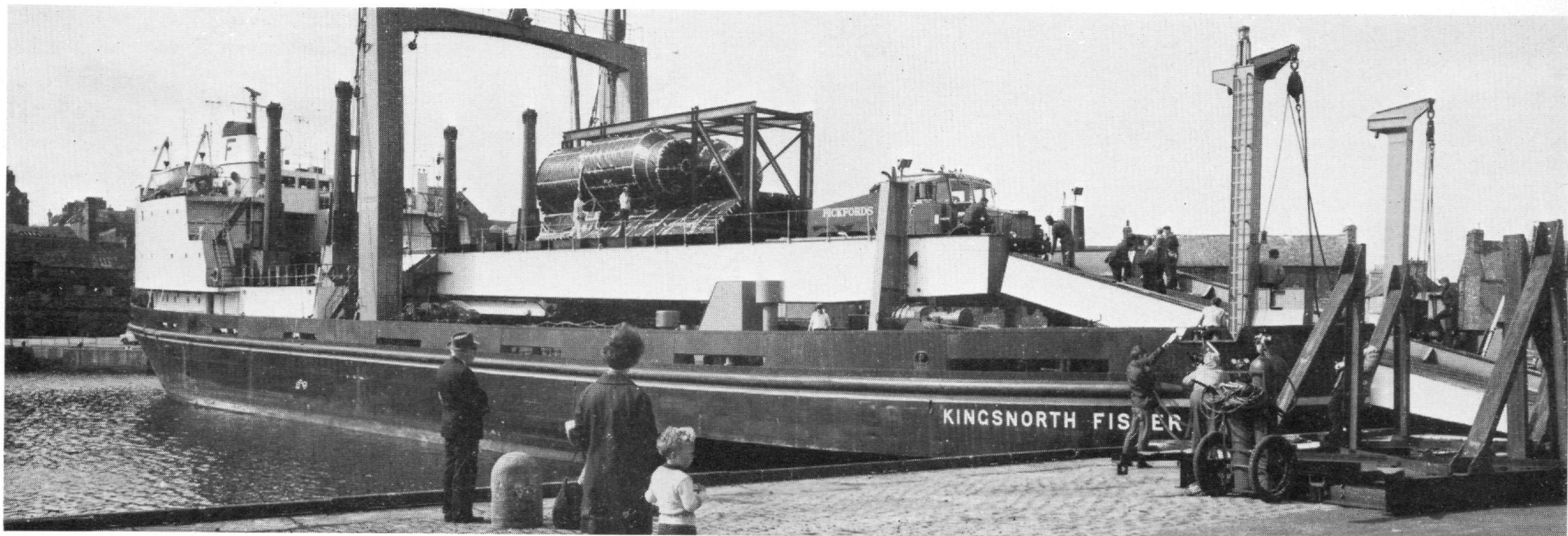
SEA ROUTE The stainless steel reactor jacket for the Prototype Fast Reactor was brought by sea from Dalmuir to Wick in Caithness and then transported by road to Dounreay. Weighing 80 tons, it was carried in four parts and assembled on site. The station is to come on power (250 megawatts) in 1971.
