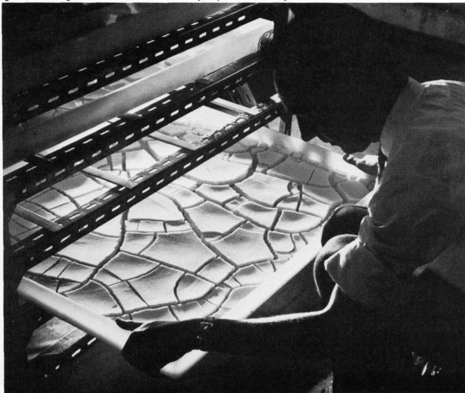
Uranium Fifty per cent of the uranium in sea-water has been recovered by a single pass through absorber beds containing granules of hydrous titanium oxide. The preparation of granules of sufficient strength to withstand long service is being studied.
