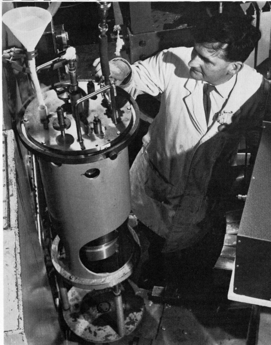
Neutron Beams Increasing use is being made of neutron beams for studying a wide range of physics problems. The instrument shown—used in association with the PLUTO reactor—investigates the magnetic disturbance caused by impurities in magnetic materials.
