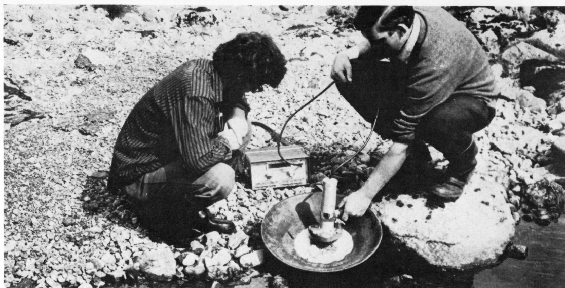
Prospecting X-ray fluorescence spectroscopy is used by the Institute of Geological Sciences for mineral prospecting. This portable analyser will assay selected elements in situ in a few seconds without chemical treatment.
