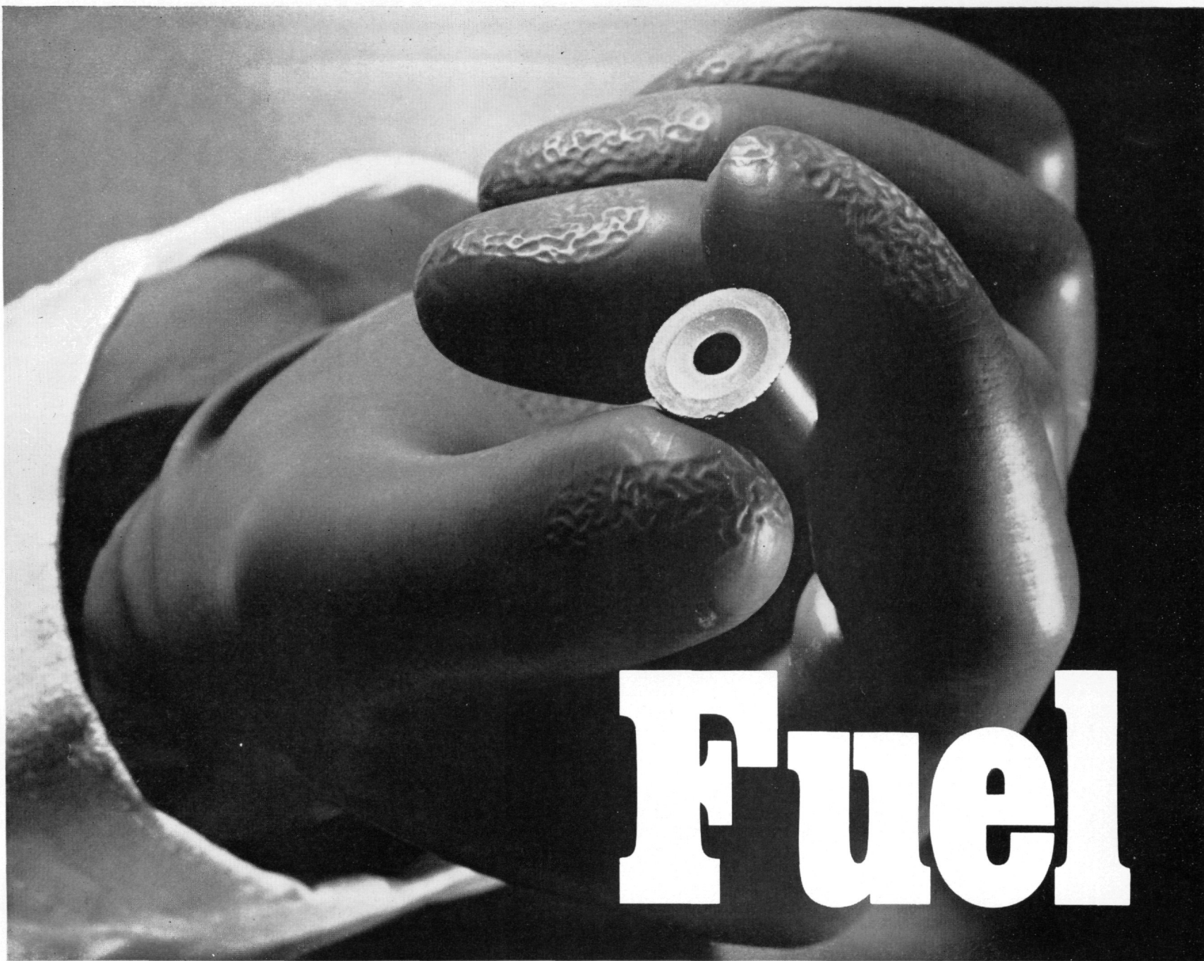
A.G.R. A uranium oxide fuel pellet for the Advanced Gas-Cooled Reactor. Each pellet will produce as much electricity as one ton of coal.
