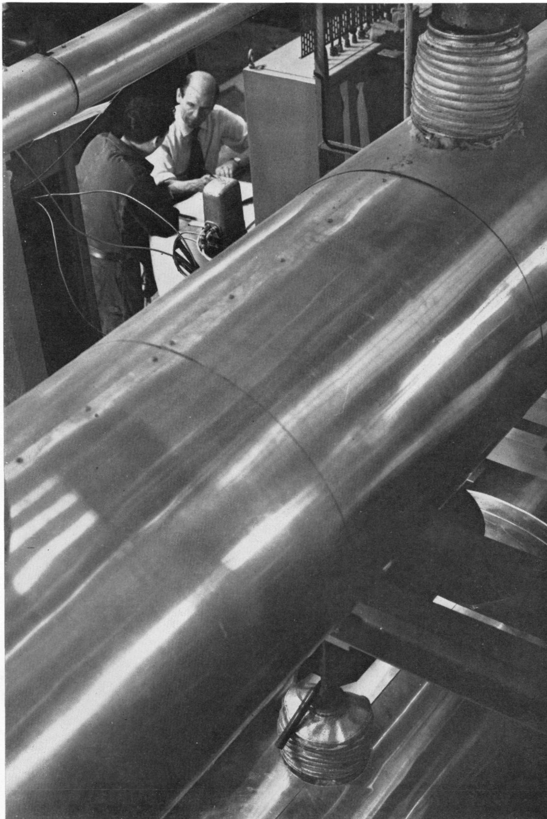
SODIUM Part of the main test loop of the 6,000 gallons-per-minute sodium pump rig at the Reactor Engineering Laboratory, Risley. R.E.L.'s main concerns are engineering, physics and instrumentation.
