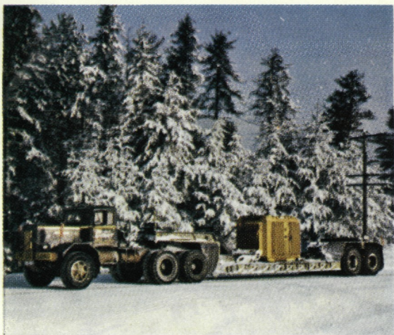
Canada: Irradiated fuel from the Canadian N.P.D. reactor en route between Chalk River and Montreal, for reprocessing at Windscale.
