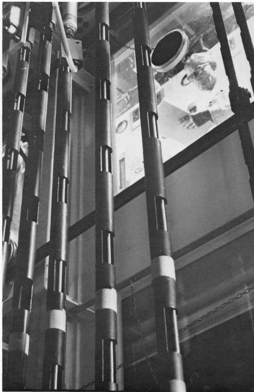
P.F.R. FUEL Manufacturing processes for the fuel of the Prototype Fast Reactor are being studied in a small-scale plant at Aldermaston (picture shows P.F.R. fuel elements in transport tubes). Construction of the 250-Megawatt P.F.R. began at Dounreay in the spring of 1966.
