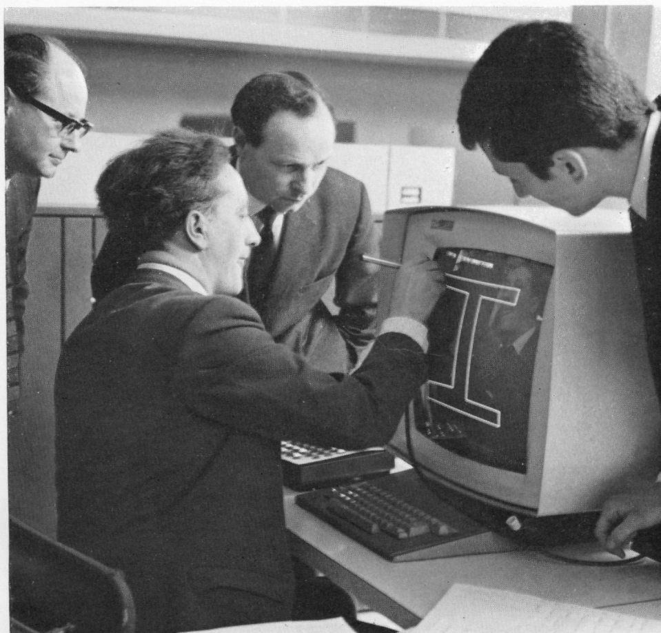
APACE staff using graphics console A project for the application of computers to engineering (APACE) began operations during the year in a small country house adjacent to Aldermaston. This project is sponsored by the Ministry of Technology to assist industry to apply modern computer aids to engineering design, planning and production, including the use of numerically controlled machine tools, and there has been a widespread response from industry seeking advice and instruction in this field.
