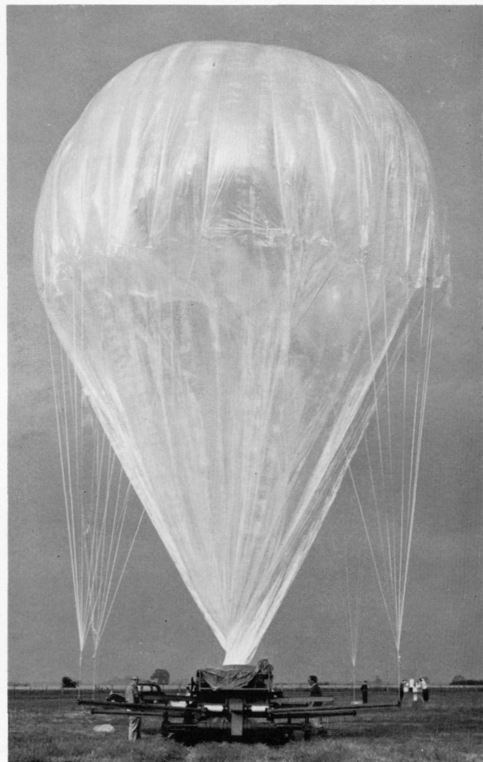
BALLOONS are cheap and effective vehicles for long duration measurements at selected stratospheric altitudes. Under a programme organised by the Science Research Council, Aldermaston manages and launches balloon flights for Bristol University. The balloons carry instruments to measure cosmic radiation.
