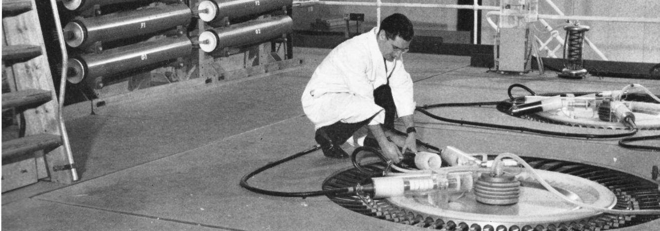
Adjustments being made to one of the sub-master switches used to fire the 996 capacitors which supply Culham with one Megajoule of energy for a large thetatron experiment.
