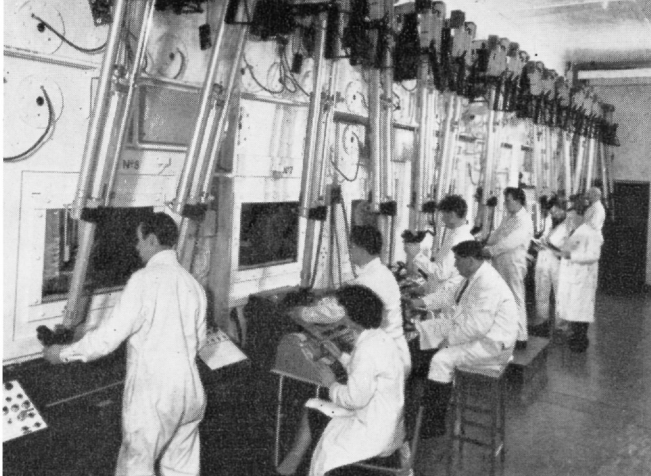
Post-irradiation examination of A.G.R. fuel elements is carried out in these "caves" adjacent to the reactor.
