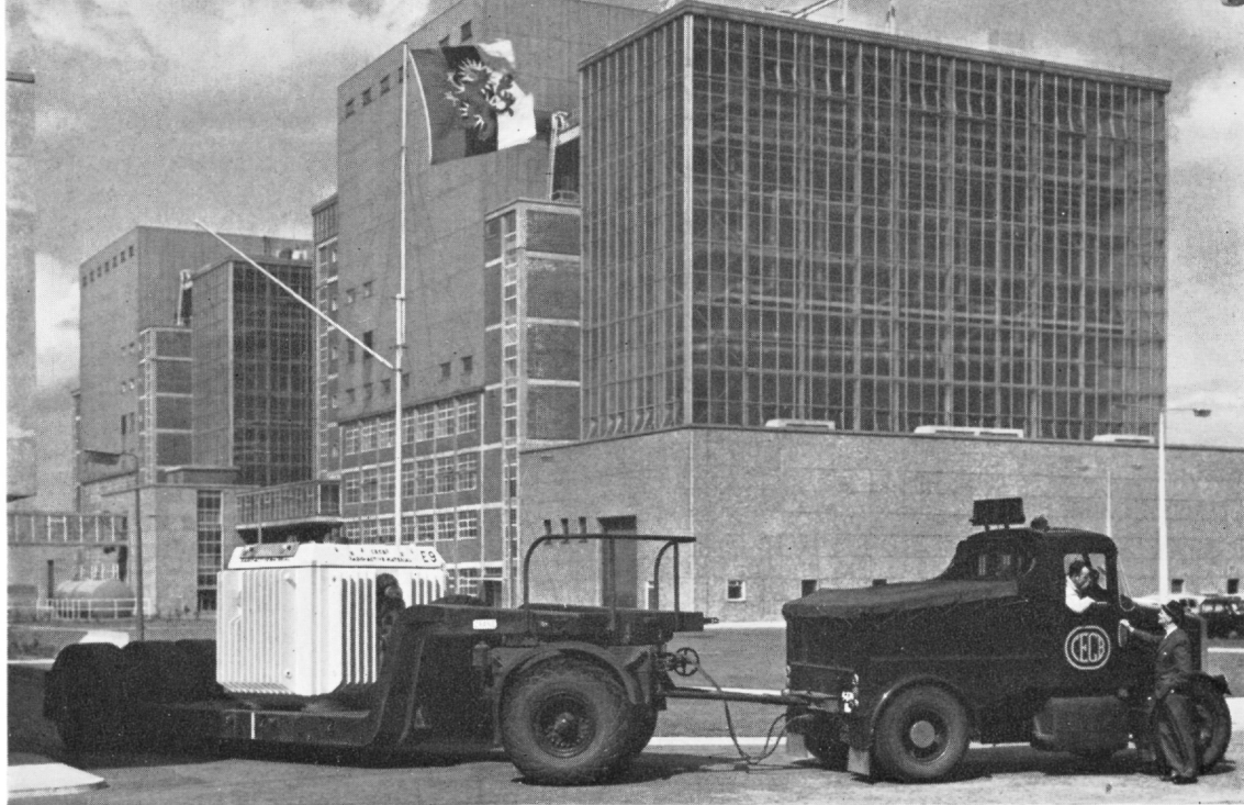
Irradiated fuel from the Bradwell power station in its transport container en route to Windscale for re-processing.
