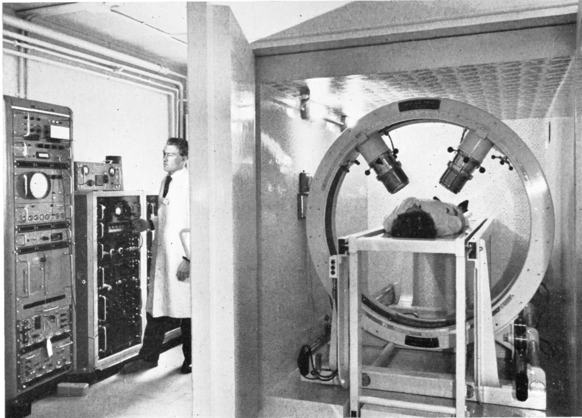
A radiation monitoring system for medical isotope investigations at Addenbrooke's Hospital, Cambridge.
