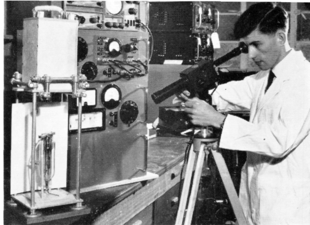
Direct conversion is an alternative to conventional electricity generation. An experimental diode under test at Harwell.
