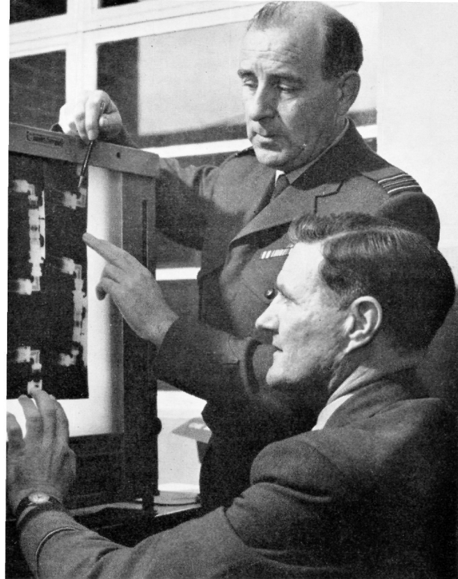
Gamma radiography is being used by the R.A.F. to check defects in aircraft.
