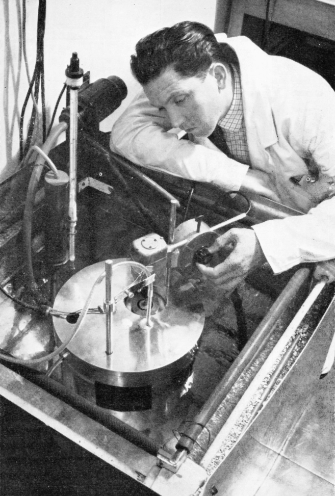
Measurement of stored energy in irradiated graphite at Culcheth.
