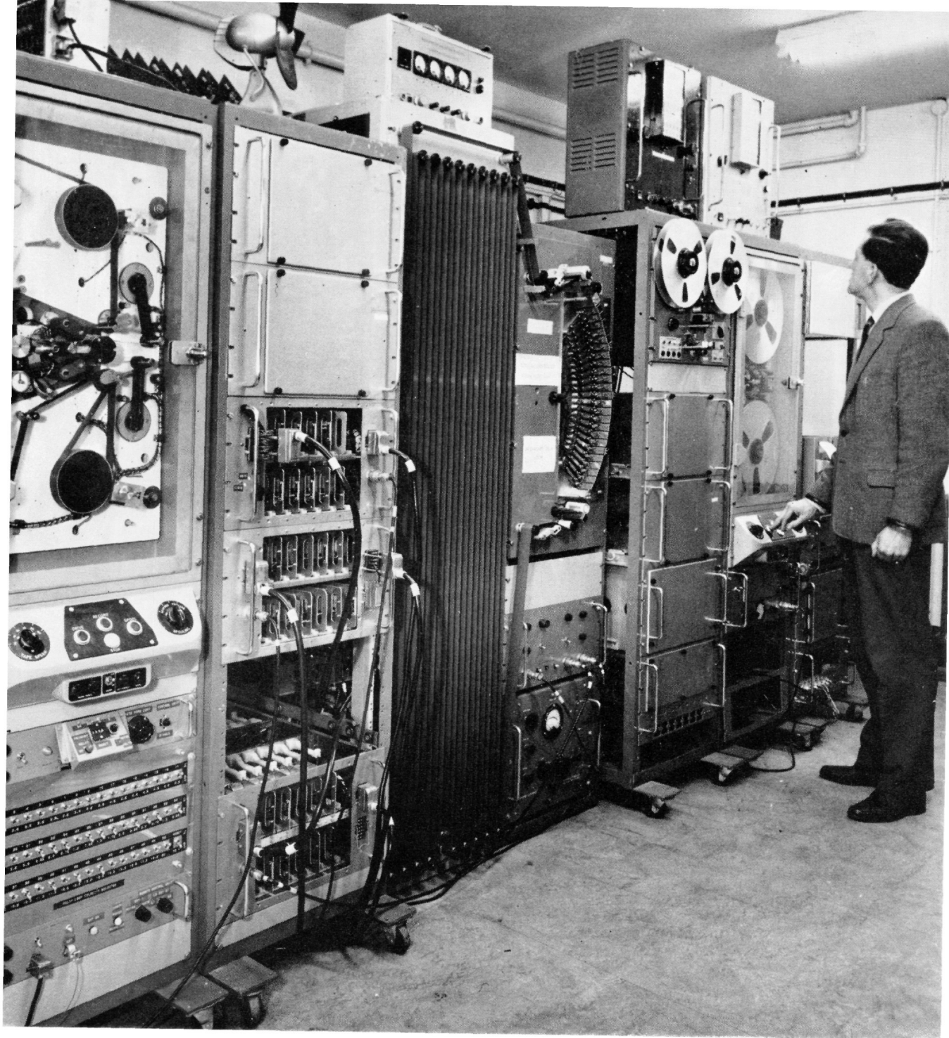
Experiments by the Weapons Group are designed to improve the ability to discriminate between earthquakes and explosions at great distances. Selected signals recorded by a large array of seismometers are processed in the magnetic tape equipment shown above before being fed into a large analogue computer.
