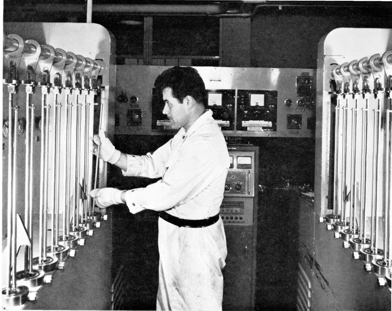
A.G.R. fuel rods being prepared for weld-testing.
