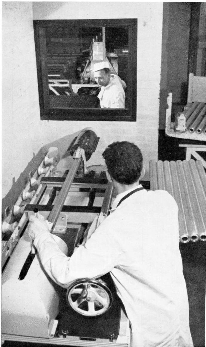
An operator (background) is fitting a uranium rod into a Calder Hall-type fuel can.
