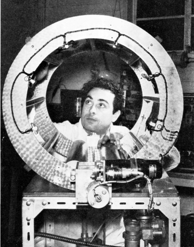
At Woolwich, apparatus is prepared before measuring very small amounts of alpha-activity in an ionisation chamber.
