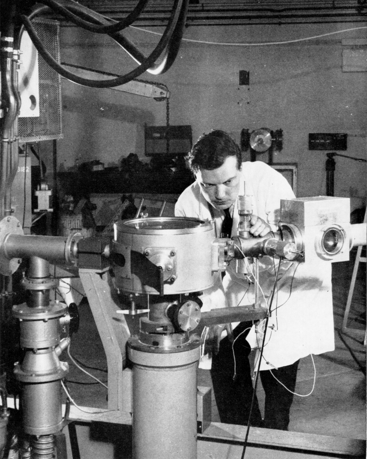
Adjusting a spectrograph which analyses particles scattered from a target bombarded by Harwell's 12 MeV tandem accelerator (used for nuclear research). Aldermaston has a similar machine.
