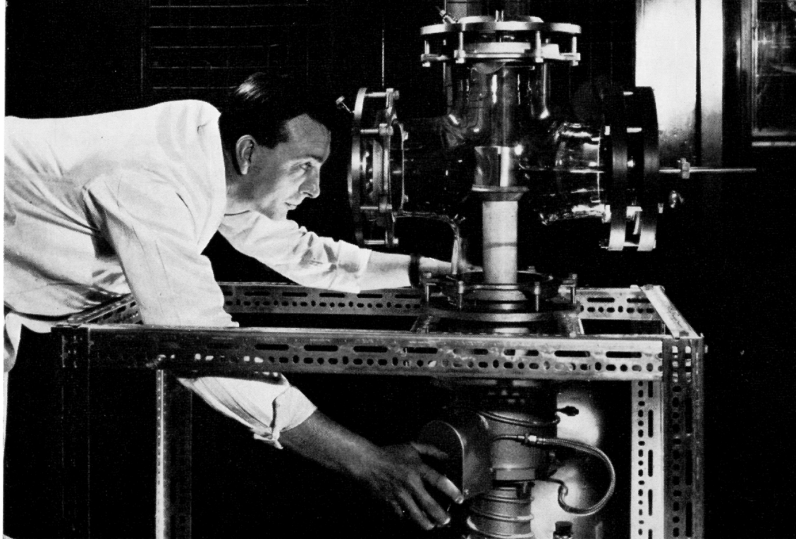
Vacuum-testing a ceramic specimen at Bracknell. The Authority are interested in ceramic fuels for power reactors.
