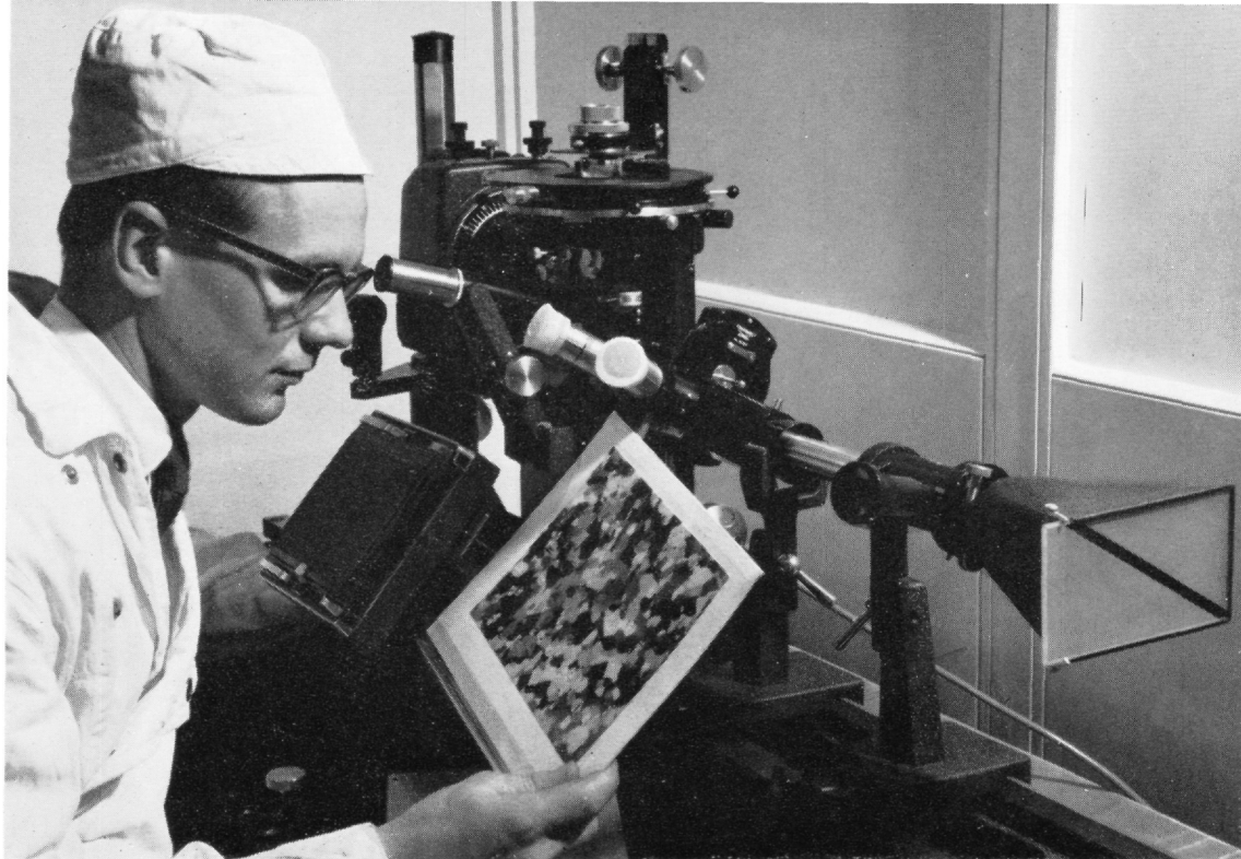
Metallographic examination of specimen of beryllium—a possible canning material for nuclear fuels.
