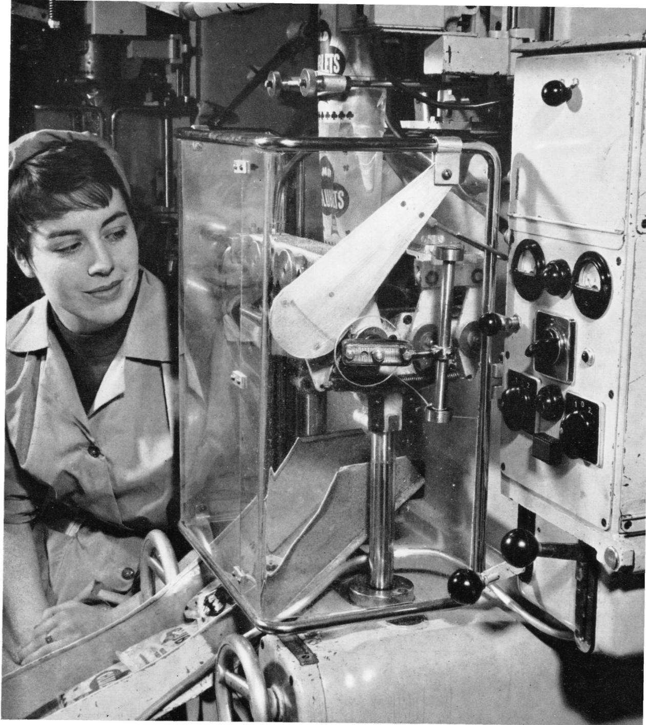
Checking Packages. Isotopes can be used to check that packages on a production line are properly filled. Photograph shows a "package monitor" in use at a biscuit factory. It does not affect the food in any way.
