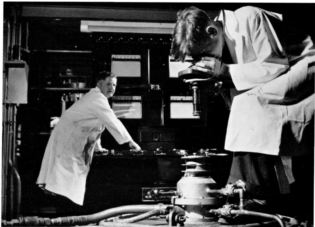
A high temperature furnace in the Harwell graphite research plant used for transforming carbon into graphite.
