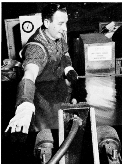
LEFT: A thickness gauge in use at the Steel Company of Wales, Velindre Works, Swansea.
