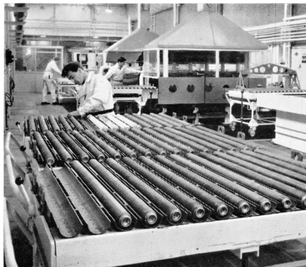
Calder Hall fuel elements in production at Springfields.
